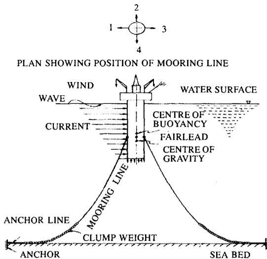
Figure 1. Schematic elevation of offshore spar platform.
