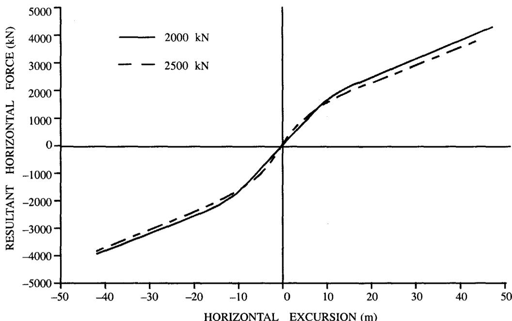
Figure 2. Resultant horizontal force–horizontal excursion for four cables for initial horizontal force
