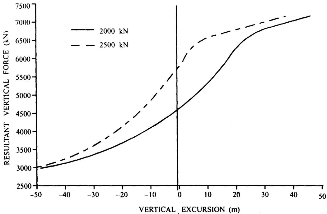
Figure 4. Resultant vertical force–vertical excursion for four cables for initial horizontal force
