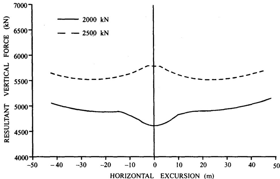
**Figure 3. Resultant vertical force–horizontal excursion for four cables for initial horizontal force**
