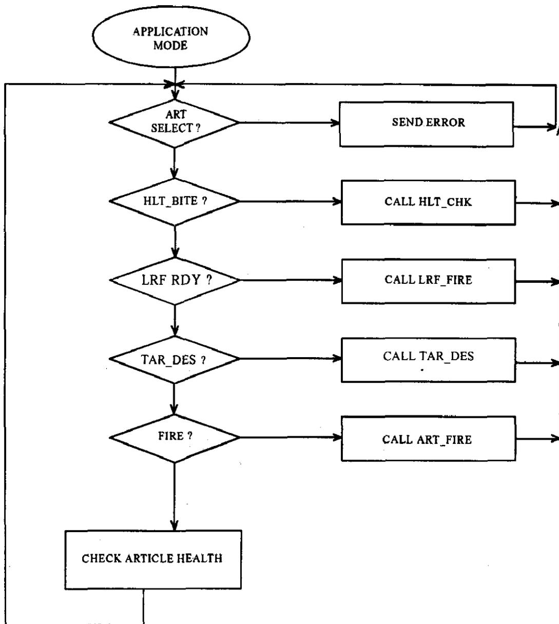
Figure 2. Application routine software flow chart
