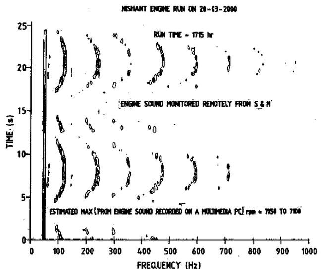
Figure 3. Spectrogram of engine sound in ground integration run.
