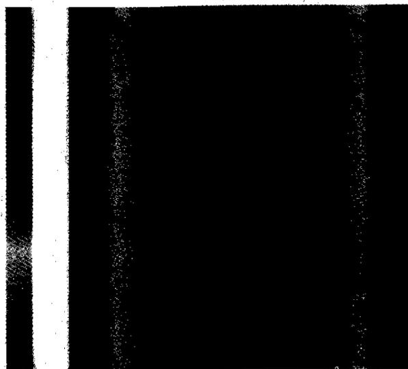
Figure 6(b). Sinogram of S4 with 100 projections vertically stacked.
