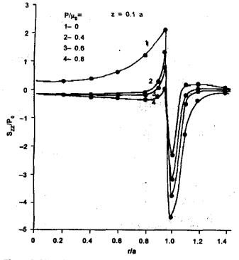
Figure 2. Variation of normal component of incremental stress s, with r.
