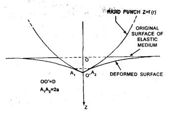
Figure 1. Indentation of a semi-infinite solid by an axisymmetrical rigid punch.
