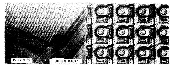
Figure 8. Part of a 2-D PbTe array with 128 x 96 pixels on an active Si chip, (a) Si substrate, (b) enlarged view of some individual pixels.
