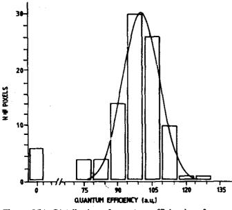
Figure 9(b). Distribution of quantum efficiencies of one arbitrary line in the 2-D array.
