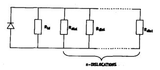
Figure 4(b). Model of the influence of dislocations on the leakage resistance.
