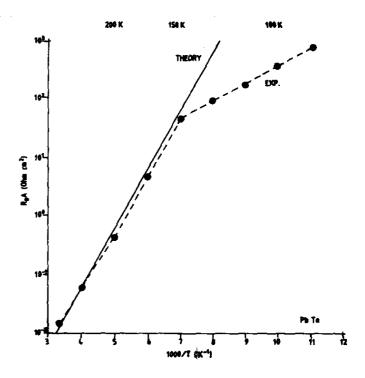
Figure 3. R<sub>o</sub>A for a *PbTe-on-Si* Schottky barrier photodiode. Cut-off wavelength at 80K is 5.5 μm. The experimental R<sub>o</sub>A products follow the calculated Schottky limit down to 150K.
