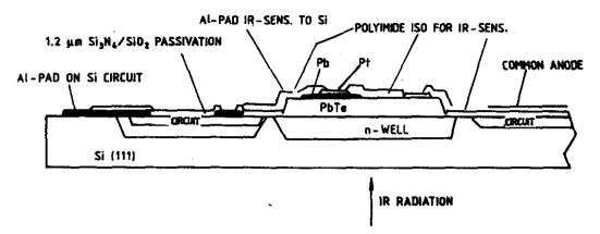
Figure 8(c). Schematic cross-section of one pixel. Each sensor is connected to an access transistor
