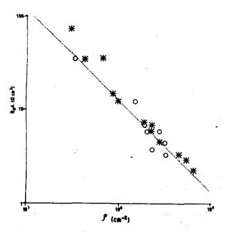
Figure 4(a). Low temperature saturation  $R_0A$  values of  $Pb_{1-x}Sn_xSe$  infrared diodes as a function of dislocation density  $\rho$ .
