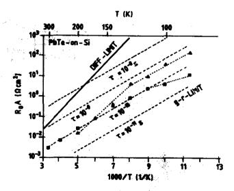
Figure 5. R<sub>0</sub>A for two *PbTe*-on-*Si* p-n<sup>+</sup> photodiode. Cut-off wavelength at 80K is 5.5 µm. The lifetimes calculated from the experimental values in *g*-*r* limit agree with the diffusion lengths limited by the dislocation densities: 5 x 10<sup>7</sup> cm<sup>-2</sup> and 1.4 x 10<sup>8</sup> cm<sup>-2</sup> for the two layers.
