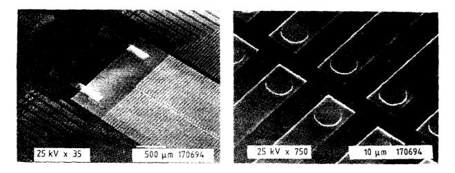
Figure 2. Partial and enlarged views of 128 x 2 Pb<sub>1-x</sub>Sn<sub>x</sub>Se-on-Si array fabricated with a batch technique. Pitch between the sensors in each line is 50 µm.
