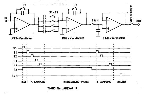
Figure 6. Schematics of the amplifier used for signal processing of each pixel. 64 of these amplifiers, together with the addressing access lines, are integrated in one read-out chip.
