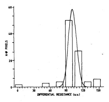
Figure 9(a). Distribution of differential resistances of one arbitrary line in the 2-D array.
