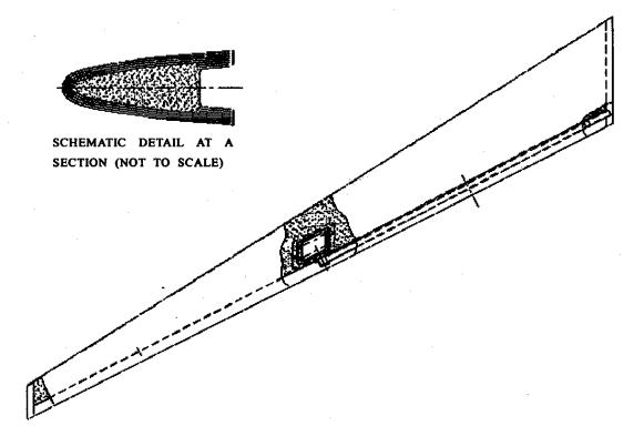
Figure 2(a). Leading edge interface of wing profile
