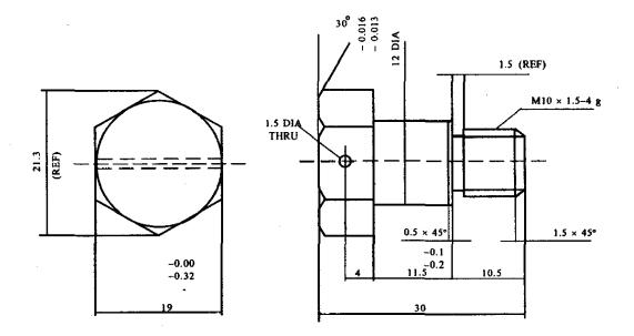
Figure 3. Wing-fuselage attachment bolt
