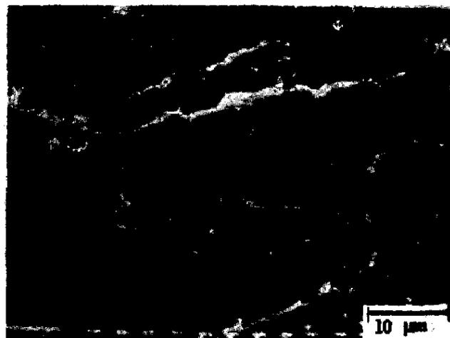
Figure 10. Tear-fractured surface of carbon black composite (mix D) at 150 °C, X400.
