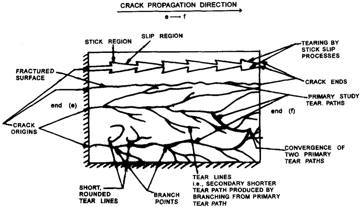
Figure 4. Line drawing showing various features observed in SEM photomicrographs
