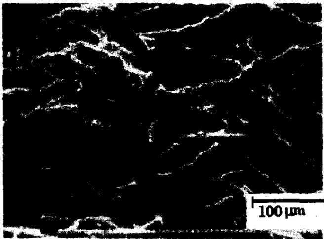
Figure 5. Tear-fractured surface of the unfilled rubber composite (mix A) at room temperature, X100.
