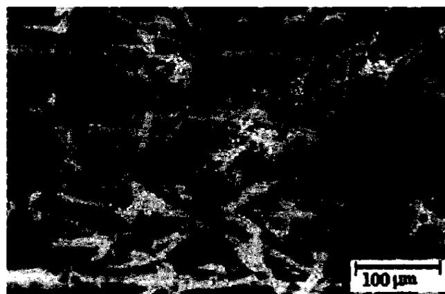
Figure 15. Tear-fractured surface of the Kevlar composite (mix C) with fibre oriented in the transverse direction at room temperature, X200.
