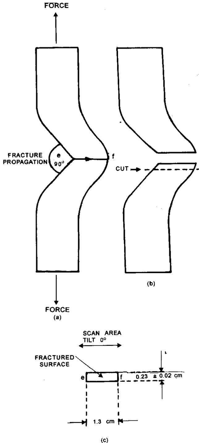
Figure 1. (a) Original test specimen (thickness  $0.23 \pm 0.02$  cm) indicates e, the point at which tear starts; f, the point at which tear ends, (b) failed specimen, and (c) scan area of the fractured surface.
