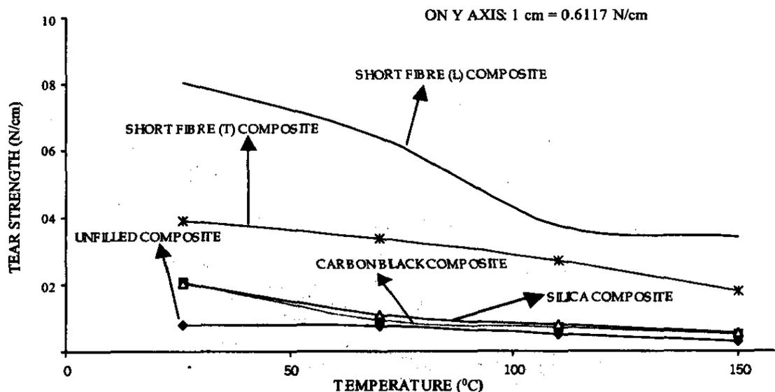
Figure 3. Plots of tear strength vs temperature. L and T are the longitudinal and transverse orientations of the fibre, respectively
