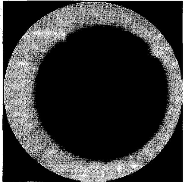
Figure 8. Reconstructed image with enlarged data for sample 2 (200 projections).
