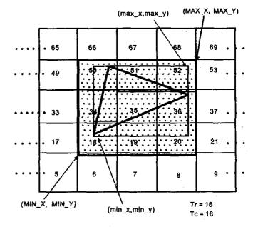
Figure 7. Enclosed rectangle of ToF
