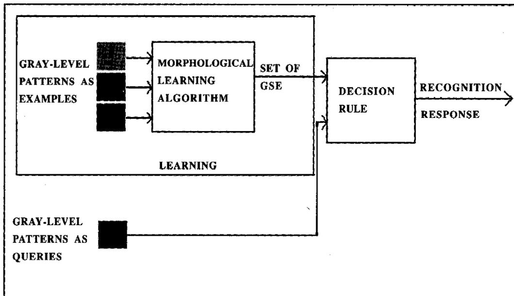
Figure 2. Block diagram of morphological learning-based object recognition method
