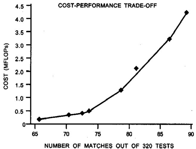
**Figure 5. Proposed algorithm allows one to trade-off performance for cost. For the 320 image test set, only about 85 had urban and/or hill features. Hence, the cost escalates rapidly as one tries to get more than 80 of the images confidently registered.**
