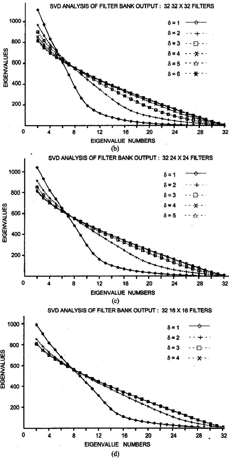
Figure 3. Analysis of various feature sets: The figures (b), (c) and (d) indicate the registration accuracy expected at PC size.  $\delta$  is the sampling rate of the input to the filter banks. The lowest value of  $\delta$  for which the graph saturates for each feature size indicates the minimum input separation required for change detection. This resolution is 4 pixels for  $32 \times 32$ , 3 pixels for  $24 \times 24$  and 2 pixels for  $16 \times 16$ .
