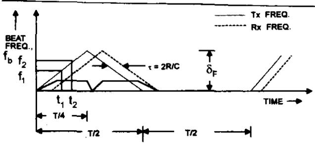
Figure 1(a). Frequency-time relationship for stationary target.
