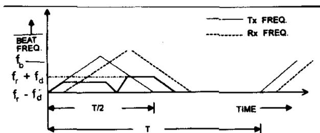
Figure 1(b). Frequency-time relationship for moving target
