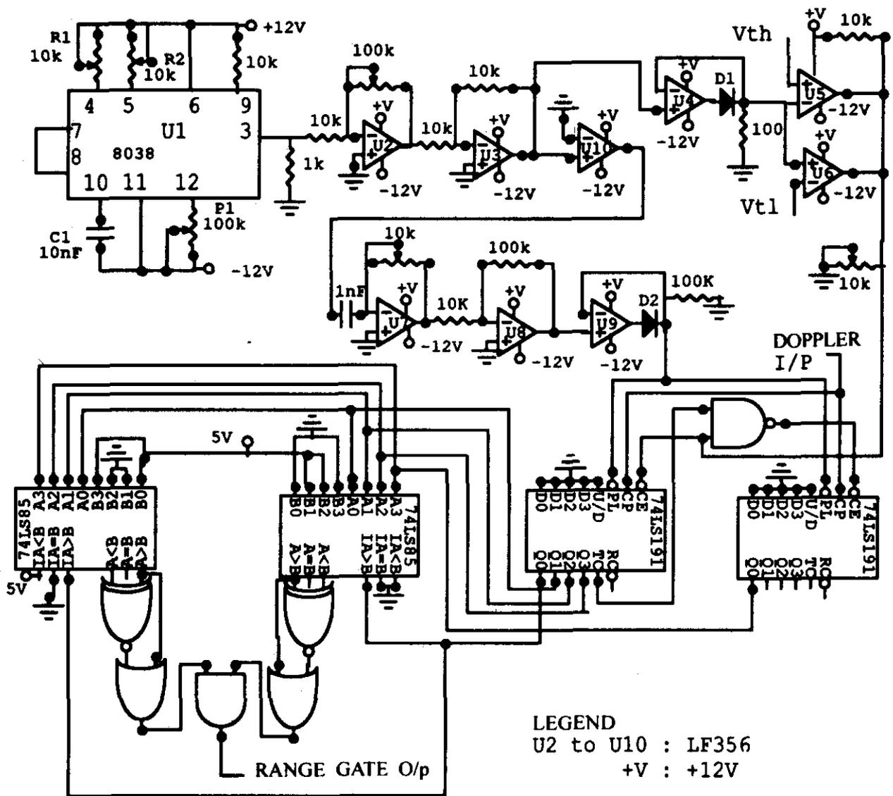
Figure 3. Hardware of the proposed range gate generator
