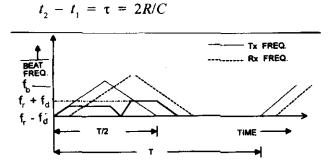
Figure 1(b). Frequency-time relationship for moving target
