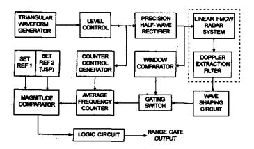
Figure 2. Schematic of the proposed range gate generator
