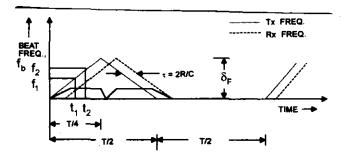
Figure 1(a). Frequency-time relationship for stationary target.
