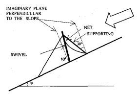
Figure 5. Swivel post inclined 10 ° uphill wrt plane perpendicular to the slope.
