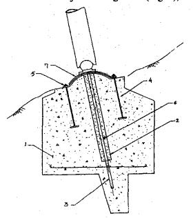
Figure 9. Swivel post with articulated ball and socket joint arrangement showing (1) concrete M-20, (2) sleeve MS, (3) anchor bolt, (4) foundation bolt, (5) nut and washer, (6) resin, and (7) base plate.
