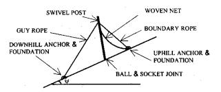
Figure 8. Main components of snow nets
