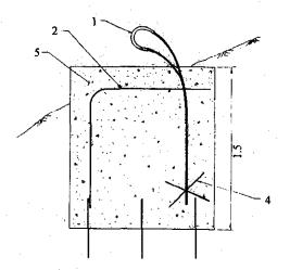
Figure 10. Uphill foundation block showing (1) anchor uphill, (2) chicken wire mesh, (3) dowel bars, (4) cross bars, and (5) concreate M20.
