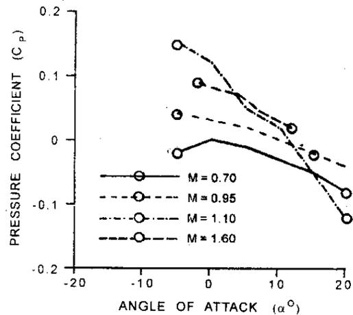
Figure 6. Effect of angle of attack ( $\alpha^\circ$ ) on pressure distribution at  $L_6$  probe location.
