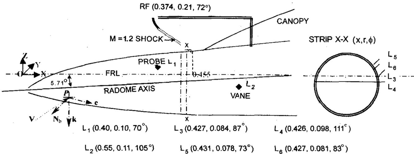
Figure 2. Schematics of front fuselage with sensor locations
