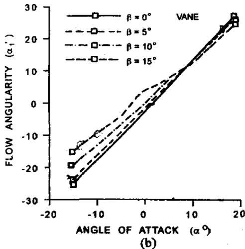
Figure 9. Flow angularity at (a)  $L_6$  probe location, and (b)  $L_2$  vane location.
