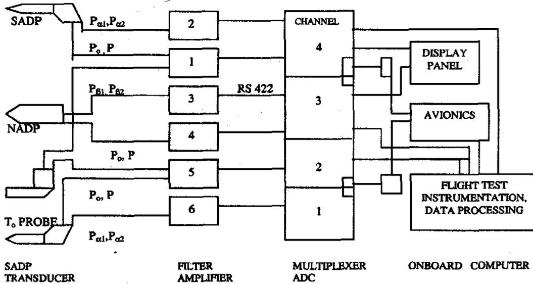
Figure 1. Data acquisition system of air data sensors
