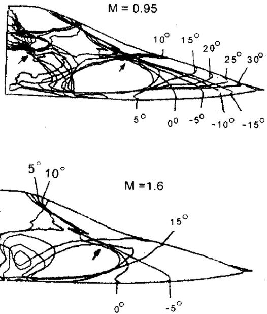
Figure 5.  $C_{p_0}$  contour lines for angle of attack ( $\alpha^\circ$ ) range at  $M = 0.95$  and  $M = 1.6$ .
