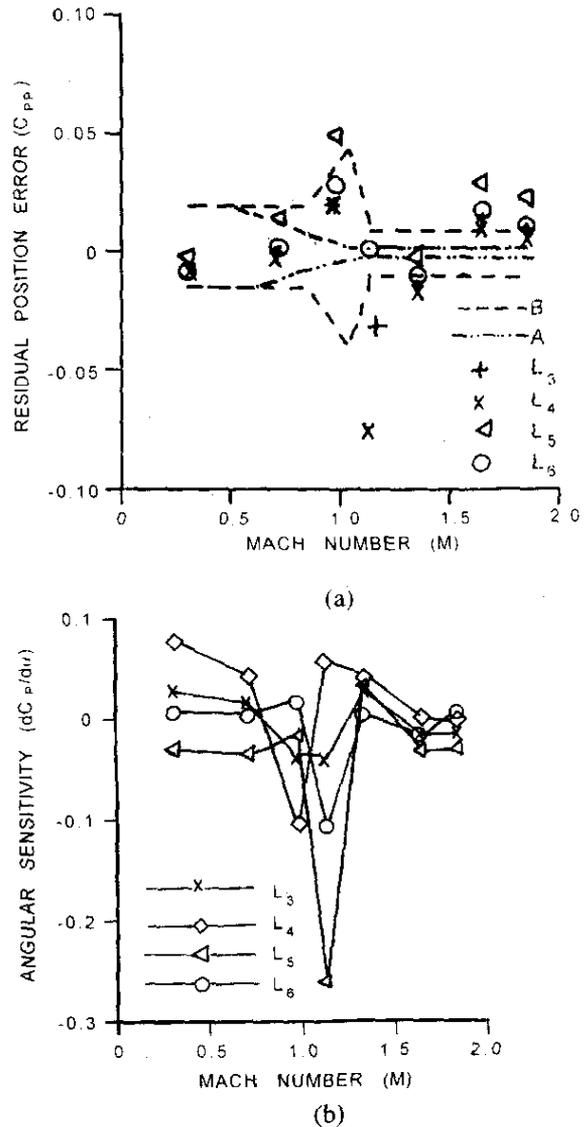
Figure 7. (a) Residual position error of probes, and (b) angular sensitivity of probes.
