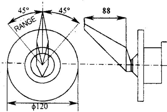
Figure 3. Angle of attack vane
