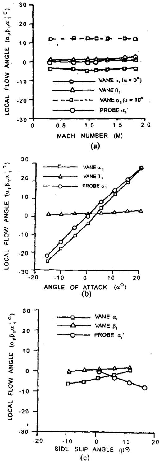
Figure 8. Variation of local angle of attack ( $\alpha_1$ ), local side slip angle ( $\beta_1$ ), and flow angularity, ( $\alpha_1'$ ) with free-stream (a) Mach Number (M), (b) angle of attack ( $\alpha^0$ ), (c) side slip angle ( $\beta^0$ ).
