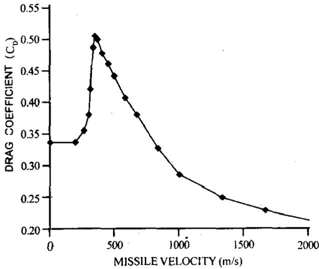
Figure 2. PRODAS-predicted drag coefficient versus velocity for missile geometry of Fig. 1.
