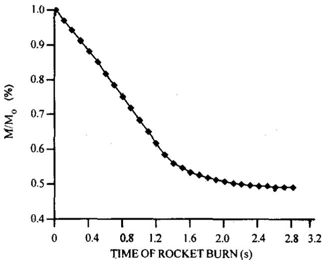
Figure 3. Change in mass versus time during rocket burn for reference missile of Fig. 1.
