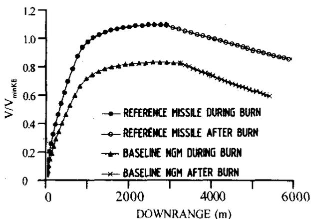
Figure 7. DIV-PRODAS-predicted trajectory for the baseline next generation missile.
