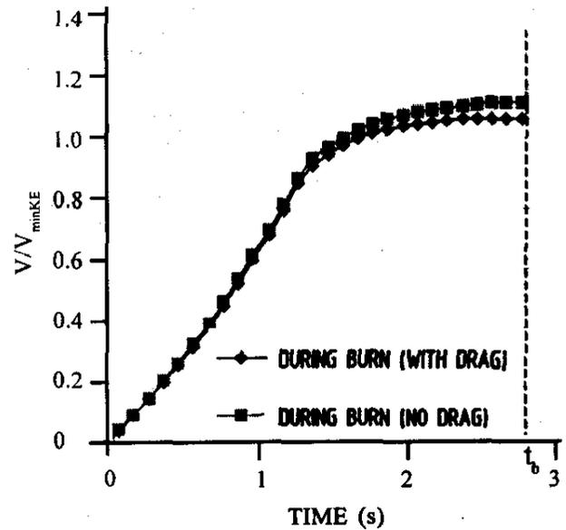
Figure 4. Predicted missile velocity versus time during rocket burn.
