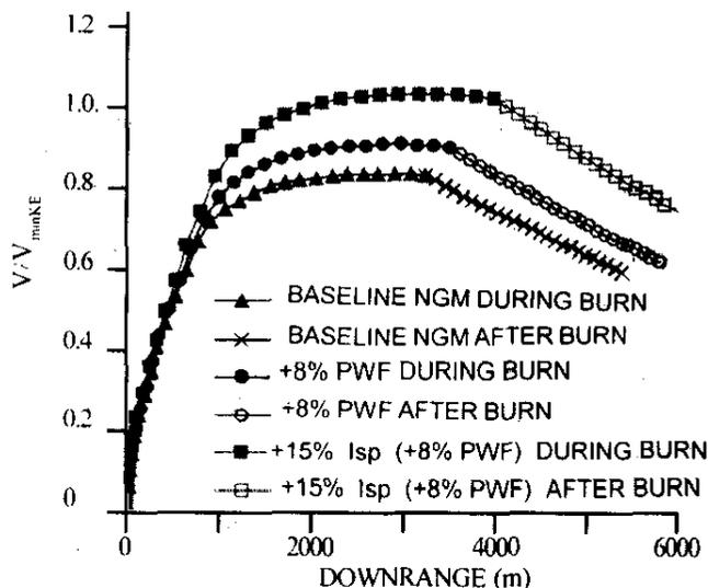
Figure 8. Effects of increased propellant weight fraction and specific impulse on next generation missile velocity.
