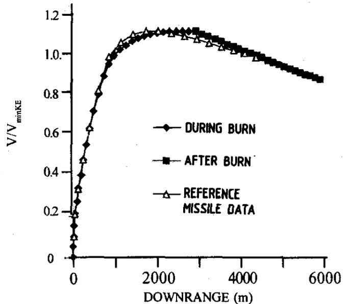
Figure 5. Validation of DIV-PRODAS-predicted trajectory for the reference missile of Figs 1-3.
