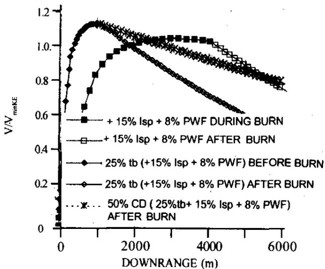
Figure 9. Effects of reduced burn time and drag coefficient on next generation missile velocity.
