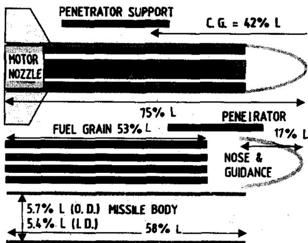
Figure 6. Lumped component illustration of a baseline next generation missile, reference to Fig. 1.
