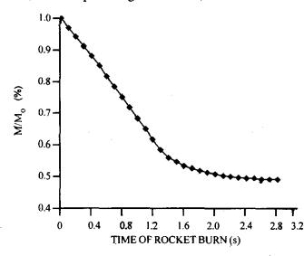
Figure 3. Change in mass versus time during rocket burn for reference missile of Fig. 1.
