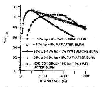
Figure 9. Effects of reduced burn time and drag coefficient on next generation missile velocity.
