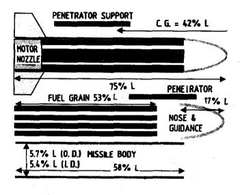
Figure 6. Lumped component illustration of a baseline next generation missile, reference to Fig. 1.
