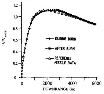
Figure 5. Validation of DIV-PRODAS-predicted trajectory for the reference missile of Figs 1-3.
