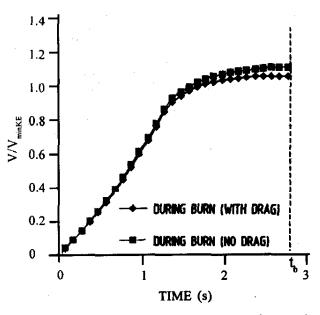
Figure 4. Predicted missile velocity versus time during rocket burn.
