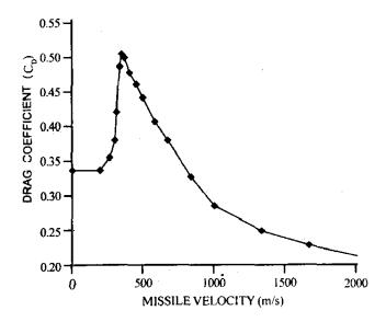
Figure 2. PRODAS-predicted drag coefficient versus velocity for missile geometry of Fig. 1.
