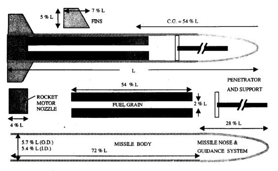
Figure 1. Lumped component depiction of a typical kinetic energy missile
