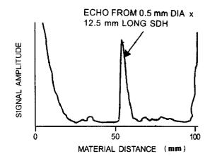
Figure 6. A-scan showing response of 0.5 mm diameter, 12.5 mm long) side-drilled hole made on 100 mm block.
