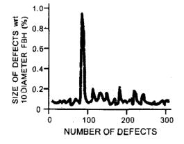
Figure 8. Equivalent size of defects observed on graphite products compared with 10 diameter FBH.
