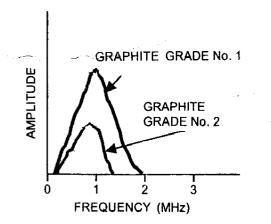
Figure 5. Ultrasonic spectroscopic response comparison on 100 mm graphite blocks (graphite grade No. 1 and grade No. 2) using 1 MHz transducers.
