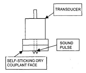
Figure 3. Transducer used with dry couplant face
