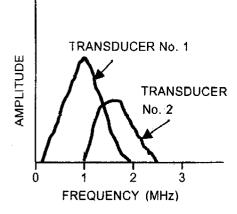
Figure 4. Ultrasonic spectroscopic response comparison on 100 mm graphite block using 1 MHz and 2 MHz transducers.
