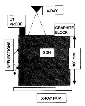
Figure 7. Side-drilled hole made on graphite block being inspected by ultrasonic technique and X-ray technique.
