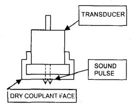
Figure 1. Transducer fitted with replaceable dry couplant face
