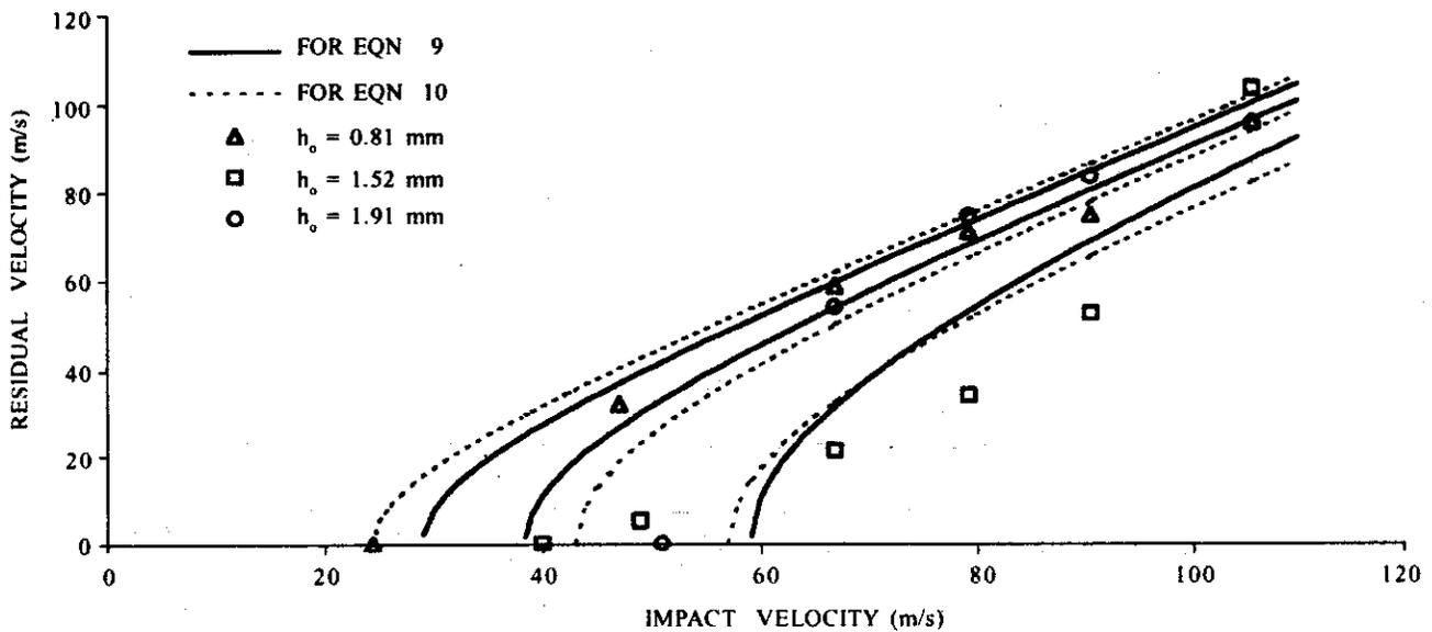
**Figure 1. Comparison of experimental residual velocity for 15° obliquity of different thicknesses of aluminium plates with the results obtained from Eqns (9) and (10).**
