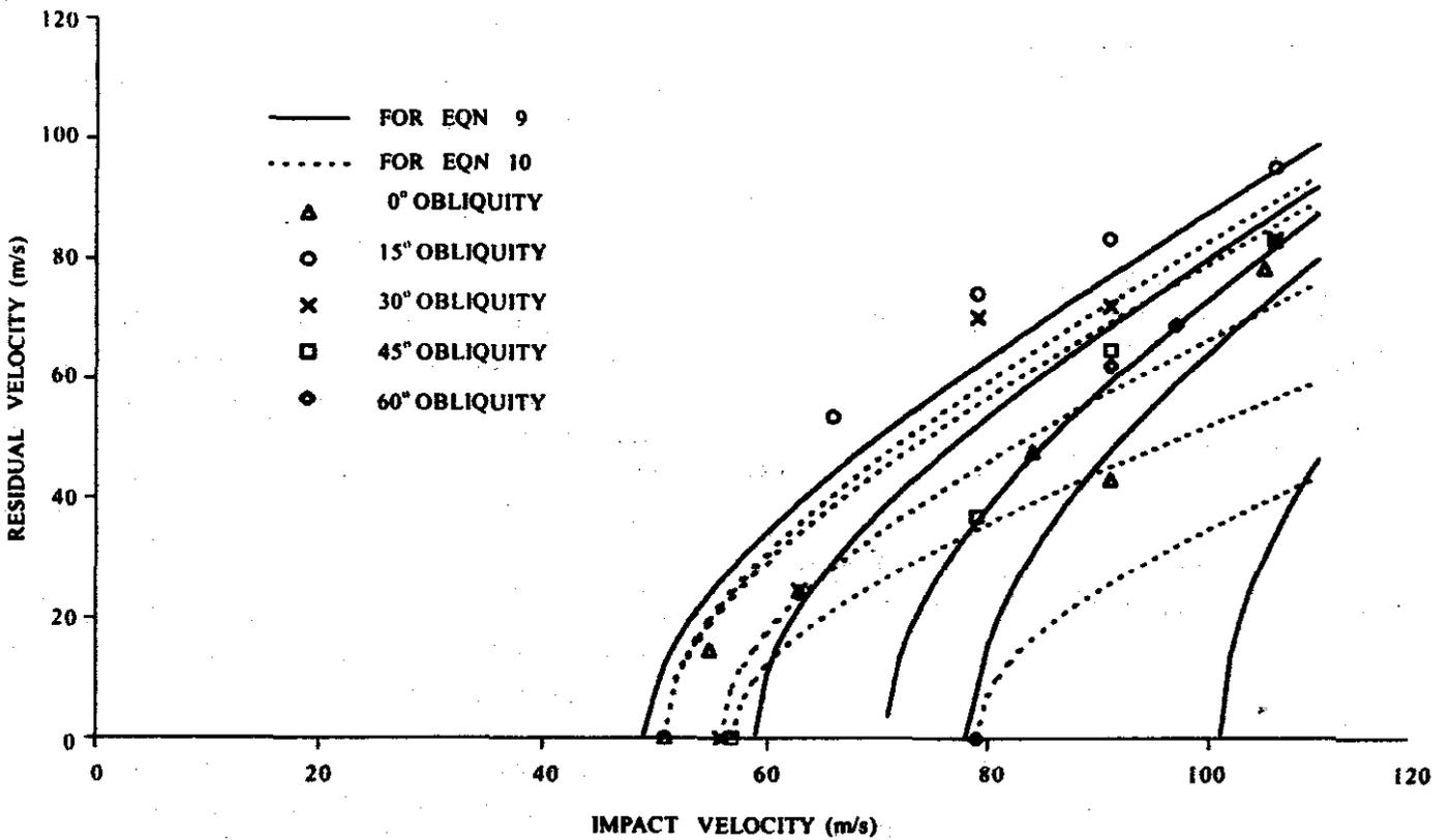
Figure 5. Comparison of experimental residual velocity for aluminium plate of 1.52 mm thickness at different angles of obliquity with the results obtained from Eqns (9) and (10).
