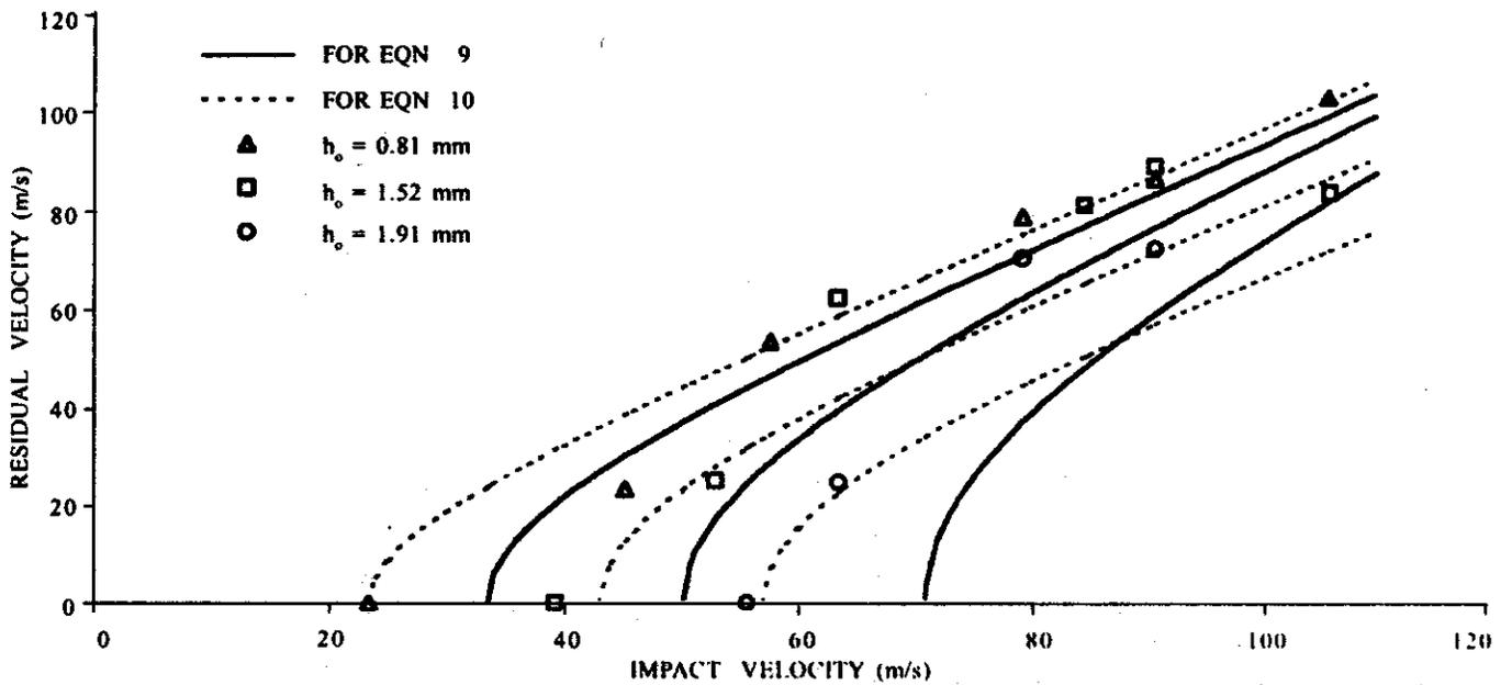
Figure 2. Comparison of experimental residual velocity for 30° obliquity of different thicknesses of aluminium plates with the results obtained from Eqns (9) and (10).
