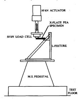
Figure 2. Test facility for evaluation of PEA elements
