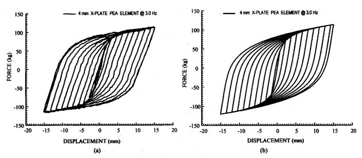
Figure 9. Comparison between theoretical and experimental results under dynamic loading at 3 Hz for a 4 mm thick X-plate PEA element: (a) Experimental curve and (b) theoretical curve.
