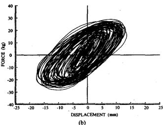
Figure 5. Typical seismic responses measured on a 4 mm thick X-plate PEA element under earthquake loading: (a) displacement-time history and (b) force-displacement curve.
