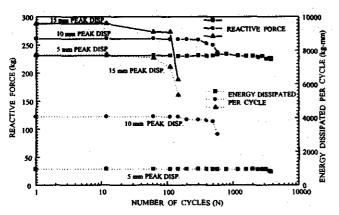
Figure 4. Dynamic test results on 6 mm thickness PEA elements at different displacement amplitudes at 3Hz.
