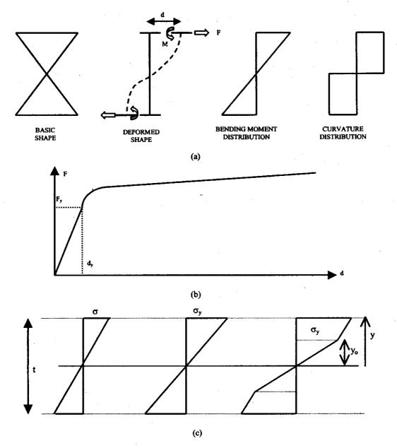
Figure 6. Analytical modelling of X-plate PEA element under static loading: (a) X-plate PEA element, (b) static forcedisplacement curve, and (c) variation of stress across thickness at various stages of loading.
