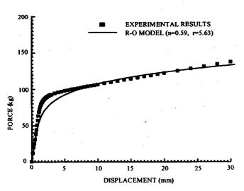
Figure 8. Comparison between theoretical and experimental results under static loading for a 4 mm thick X-plate PEA element.
