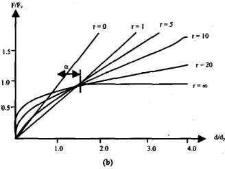
Figure 7. Ramberg-Osgood model employed for modelling X-plate PEA elements under dynamic loading:
