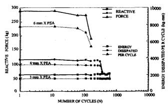
Figure 3. Dynamic test results on different PEA elements at constant peak displacement amplitude of 15 mm at 3 Hz.
