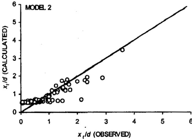
Figure 2. Observed and predicted penetration depth (model 2).
