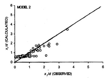
Figure. 2 Observed and predicted penetration depth (model 2).
