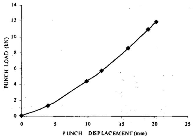
Figure 6. Curve of punch load versus punch displacement.
