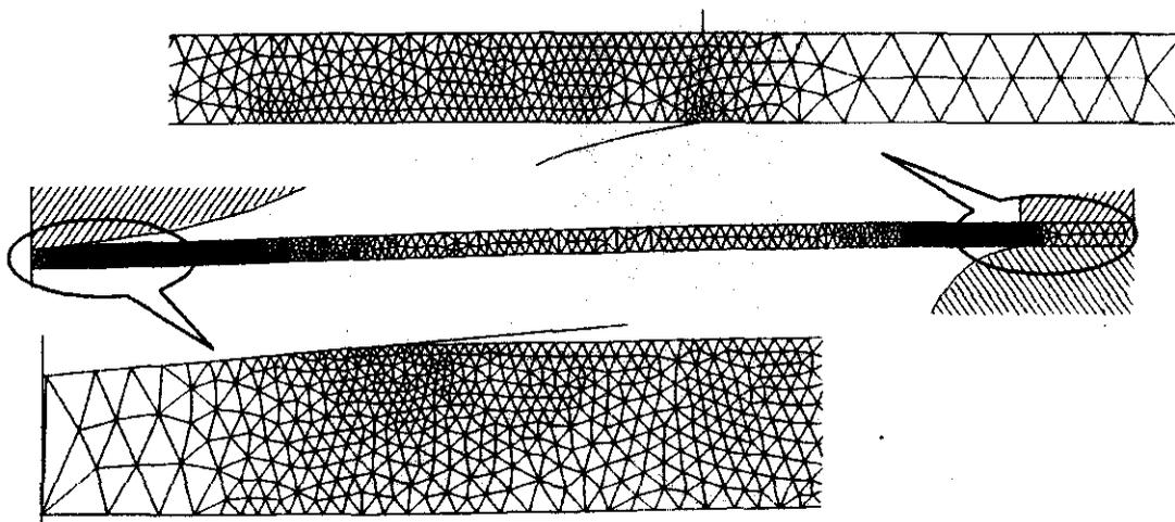
Figure 3. Mesh at punch displacement of 2.5 mm
