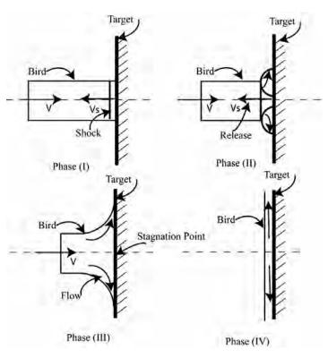
Figure 2. Different stages of bird impact<sup>3</sup>.
