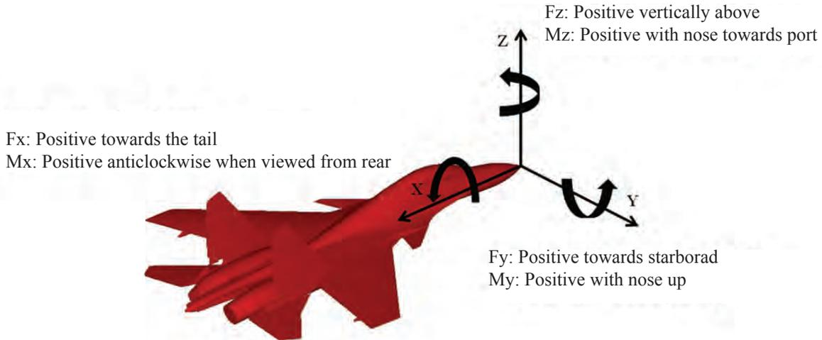
Figure 4. Sign convention for aerodynamic forces and moments.
