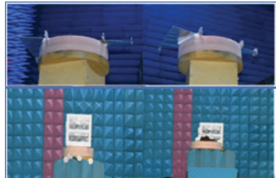
Figure 4. Target with a chaff cloud is placed on the upper surface of a turntable.
