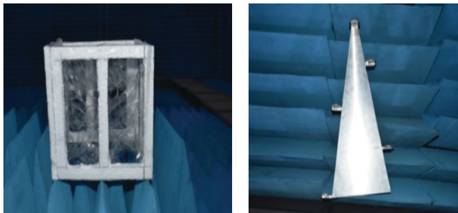
Figure 2. Scaled-down model of the chaff cloud (30 cm x 30 cm x 30 cm) and target.
