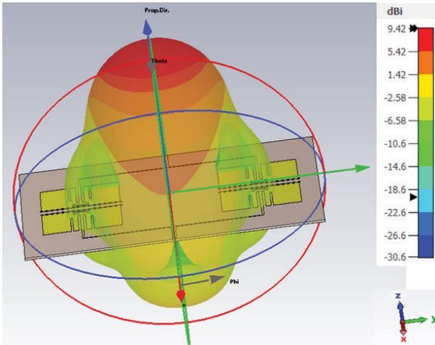
Figure 6. 3-D gain of the proposed IBFD antenna system under Tx port excitation, while the Rx port is terminated with 50 Ω matched load at 3.5 GHz.
