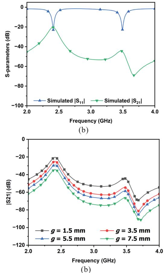
Figure 4. (a) Simulated S-parameters of the designed dual band IBFD antenna array system, (b)  $|S_{21}|$  of the proposed IBFD antenna system for different values of design parameter gap  $g$ .
