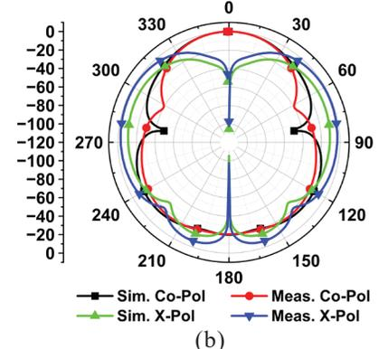
Figure 10. Far-field radiation pattern of the proposed IBFD antenna under Tx port excitation, while the Rx port is terminated with 50  $\Omega$  matched load at 3.5 GHz in (a) xoz-plane (b) yoz-plane.
