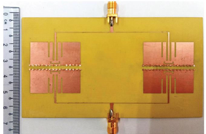
Figure 7. Fabricated prototype of the proposed IBFD antenna array system.
