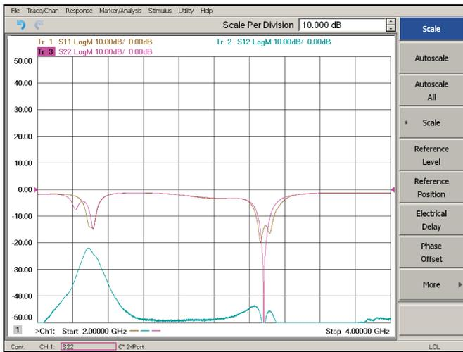
Figure 8. (a) Measured S-parameters of the designed dual band IBFD antenna array system, (b) Measurement of prototype using VNA (c) Snap of VNA screen.
