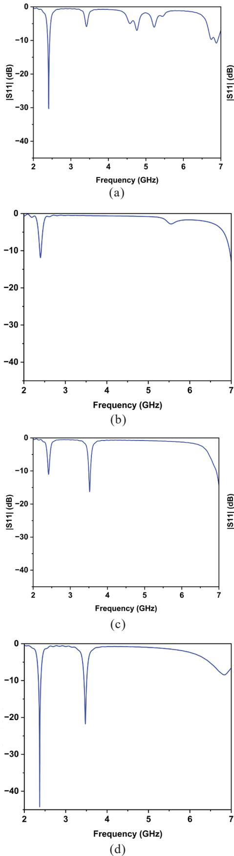
Figure 3. S-parameters of different stages of unit element shown in Fig. 2 (a) MPA-I, (b) MPA-II, (c) MPA-III, and (d) MPA-IV.
