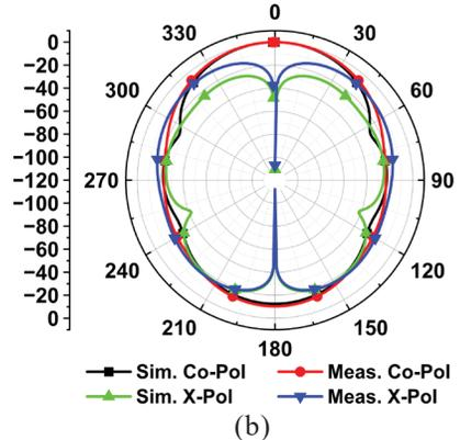
Figure 9. Far-field radiation pattern of the proposed IBFD antenna under Tx port excitation, while the Rx port is terminated with 50  $\Omega$  matched load at 2.4 GHz in (a) xoz-plane (b) yoz-plane.
