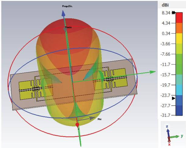
Figure 5. 3-D gain of the proposed IBFD antenna system under Tx port excitation, while the Rx port is terminated with 50 Ω matched load at 2.4 GHz.
