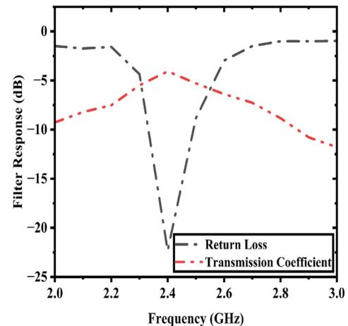
Figure 4. Filter response of the presented filtenna.
