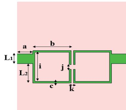
Figure 3. Filter design of the filtenna.
