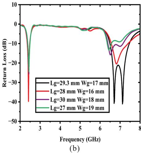
Figure 5. (a) Parametric analysis using different substrates; and (b) Parametric analysis varying length and width of the ground plane.
