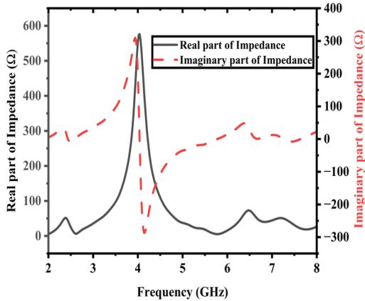
Figure 8. Impedance of the suggested design.
