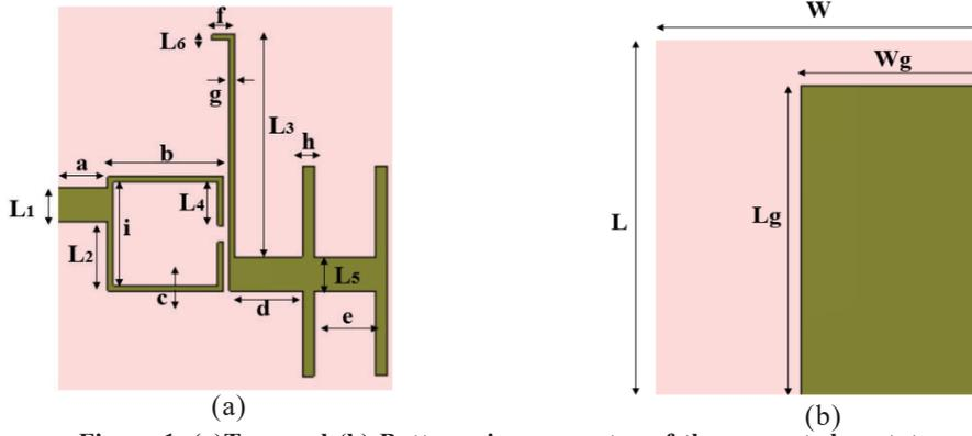
Figure 1. (a)Top; and (b) Bottom view geometry of the suggested prototype.
