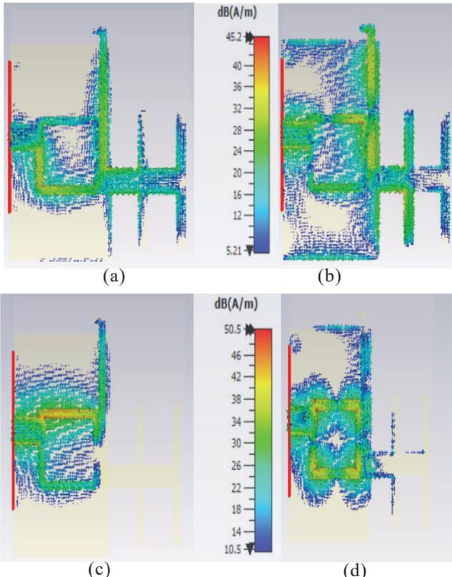
Figure 9. Surface currents of the filtenna at (a) 2.4 GHz; (b) 7.2 GHz; (c) 3 GHz; and (d) 10 GHz.
