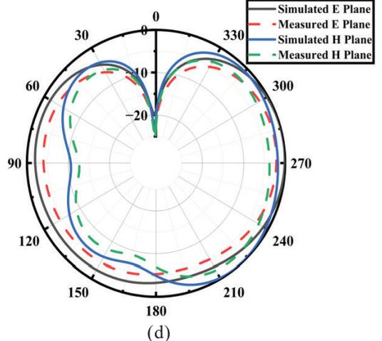
Figure 10. (a) Gain of the suggested filtenna; (b) Measurement setup for computing radiation pattern; (c) Far field patterns of the suggested filtenna at 2.4 GHz; and (d) 7.2 GHz.
