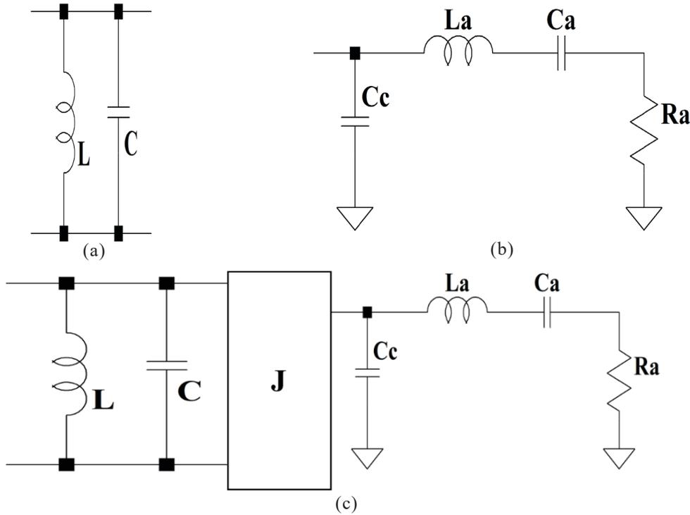
Figure 2. (a) Circuit modelling of square open loop resonator; (b) Circuit modelling of the H shaped radiator; and (c) Circuit modelling of the proposed filtering antenna.
