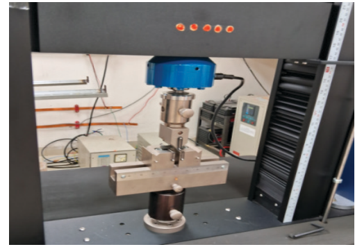
Figure 6. Set up for flexural test.
