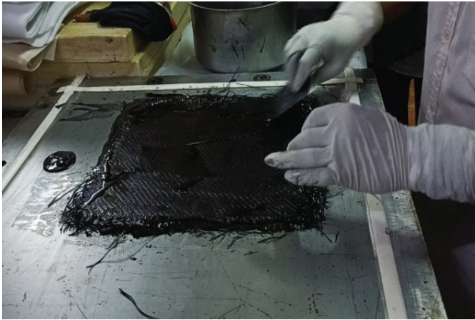
Figure 2. Hand lay-up process.
