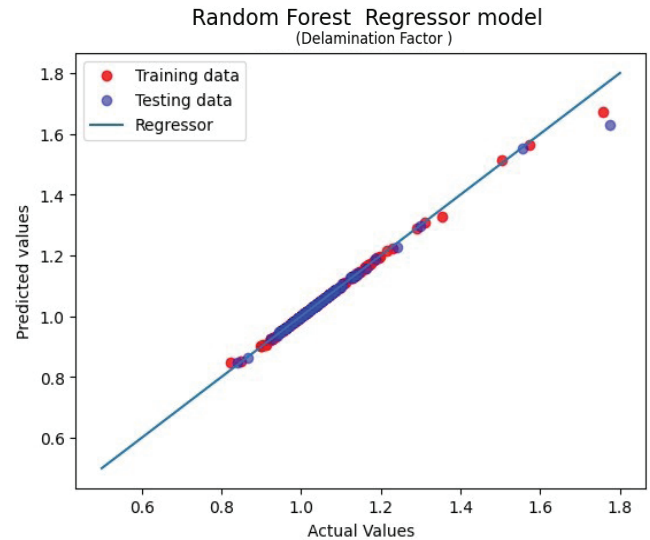
Figure.7 Actual Vs predicted delamination-RF.
