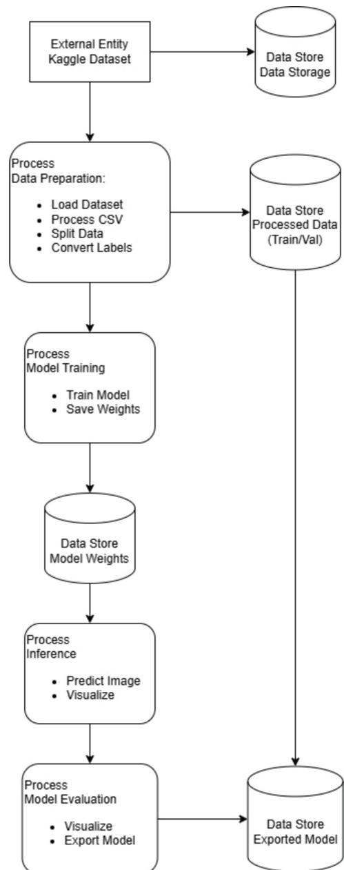
Figure 1. Flow diagram of the proposed model.
