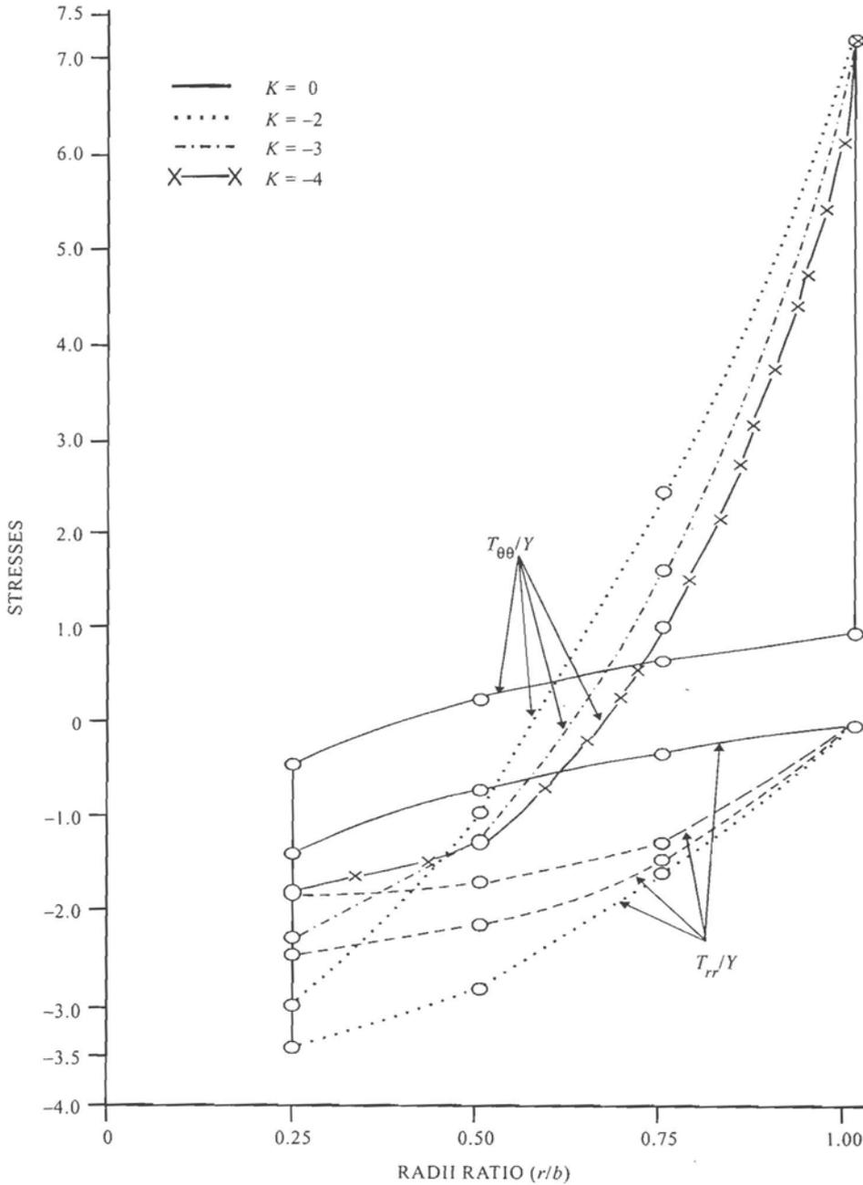
Figure 1. Plastic stress distribution in a non-homogeneous circular cylinder under internal pressure
