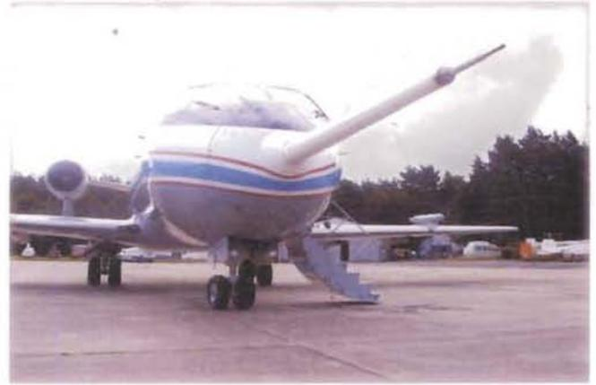
Figure 1. ATTAS aircraft with 5-hole probe
