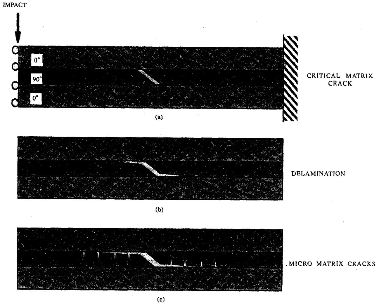
Figure 1. Failure mechanism in a layered composite
