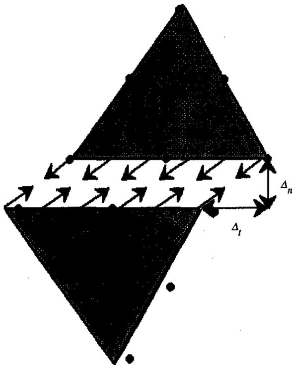
Figure 2. Illustrating the concept of the cohesive/volumetric finite element technique.
