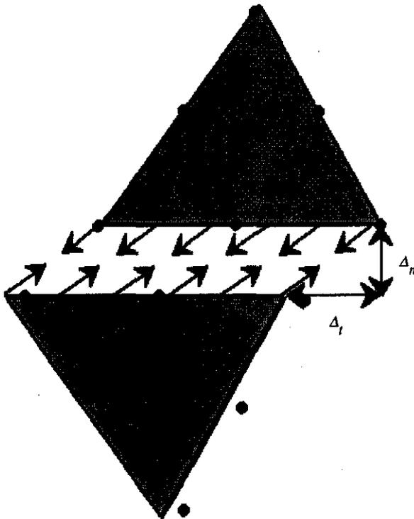
Figure 2. Illustrating the concept of the cohesive/volumetric finite element technique.
