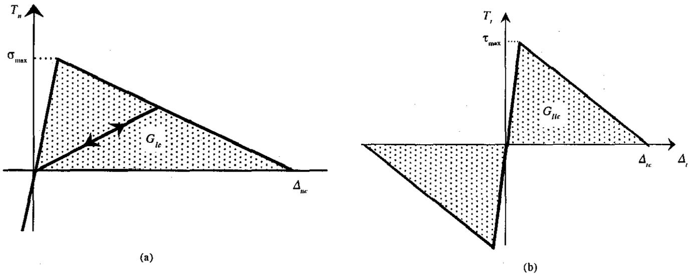
Figure 3. Cohesive law for (a) pure tension and (b) pure shear
