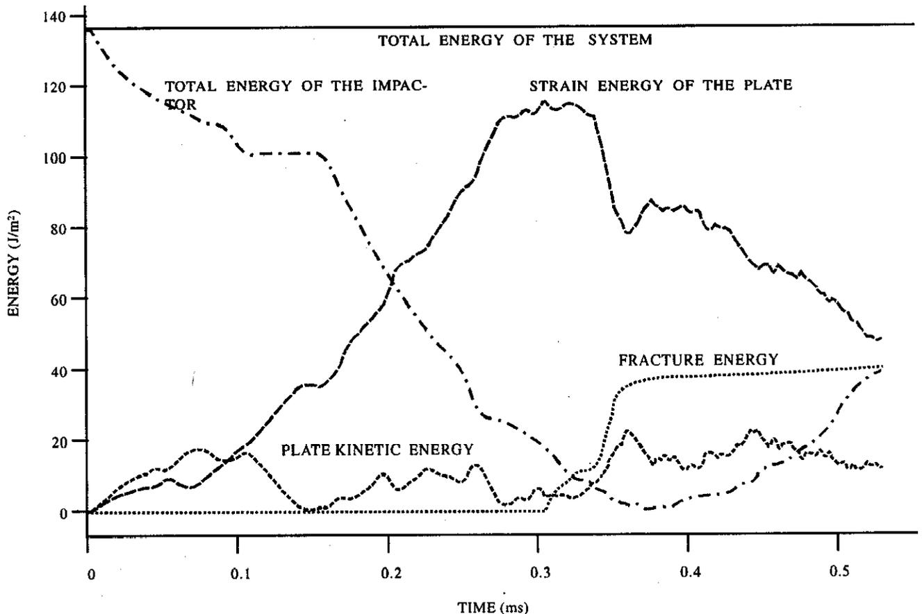
Figure 6. Evolution of energy of the impacted plate
