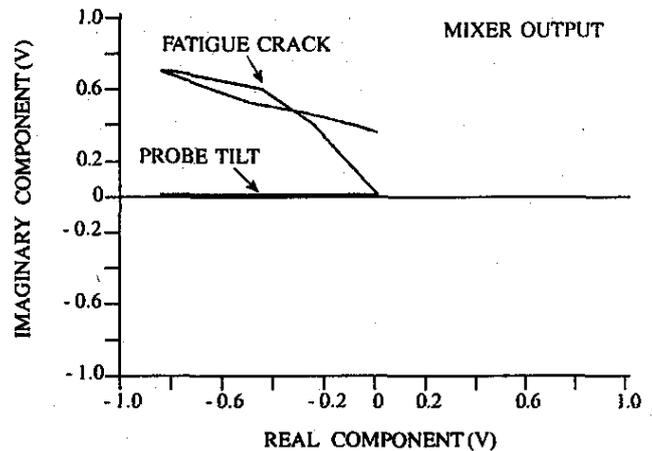
Figure 7. Eddy current signal from reference crack of 4 mm length after dual-frequency mixing.
