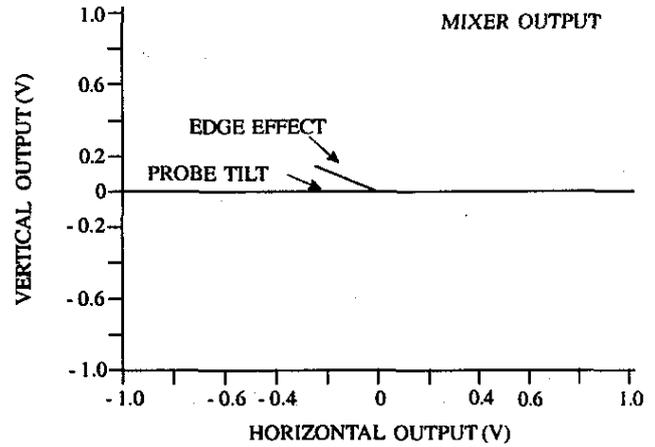
Figure 6. Eddy current signal from probe tilt and edge effect after dual-frequency mixing.
