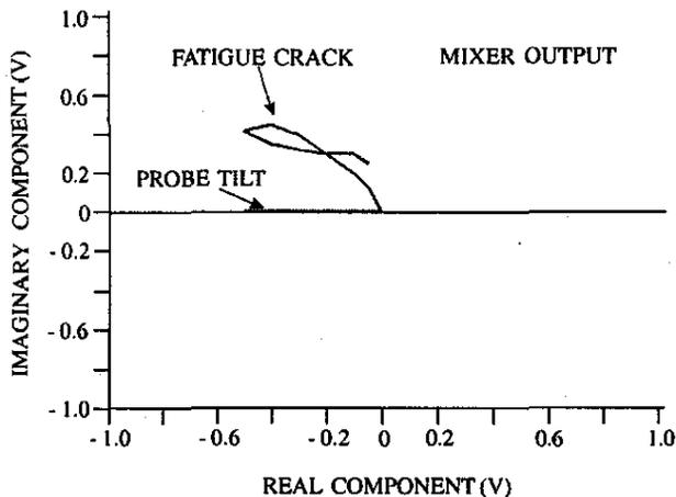
Figure 8. Eddy current signal for a crack of 2 mm length in the compressor disc detected by dual-frequency mixing method.
