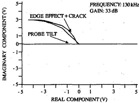
Figure 5. Eddy current signal at 130 kHz for the reference crack of 4 mm length along with signal due to edge effect and probe tilt.
