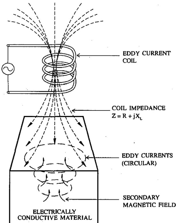
Figure 1. Principle of eddy current testing
