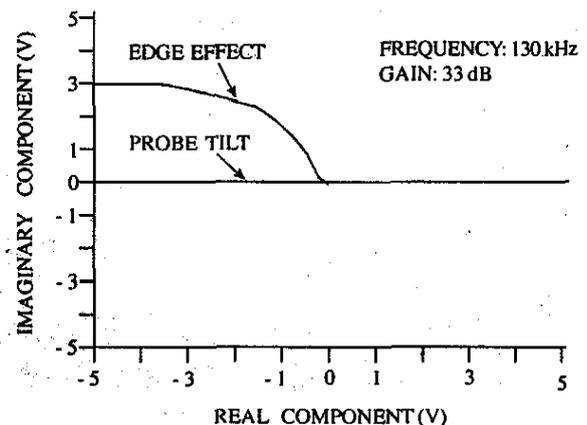
Figure 4. Eddy current signals from probe tilt and edge effect at 130 kHz.
