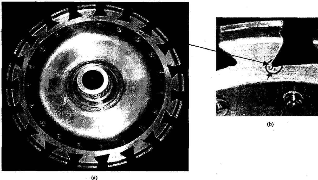
Figure 2. Aero engine compressor disc: (a) with a surface crack of 4 mm length in the dovetail region and (b) close view of the crack originating from the dovetail region.
