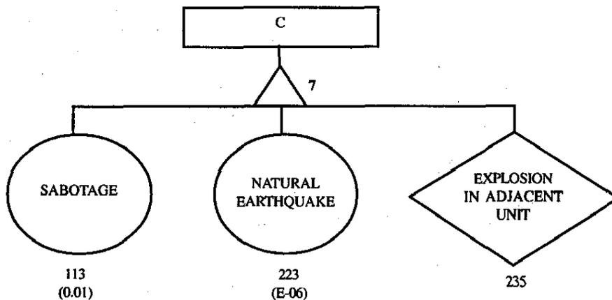
Figure 1(d). Fault tree for the release of HCl from the storage tank
