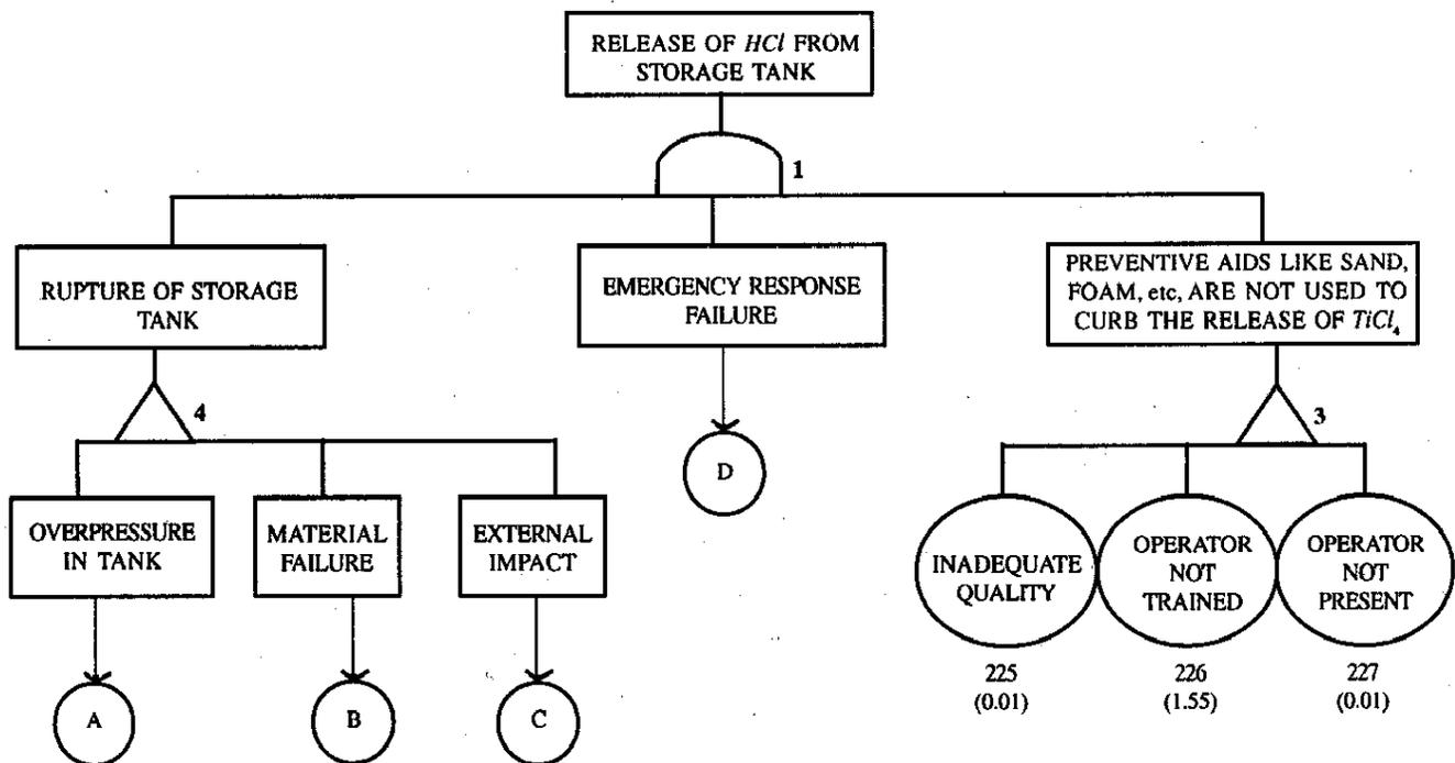
**Figure 1(a). Fault tree for the release of *HCl* from the storage tank**
