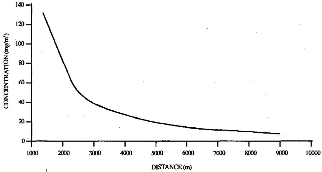
Figure 3. Variation of concentration with distance (up to TLV limit)
