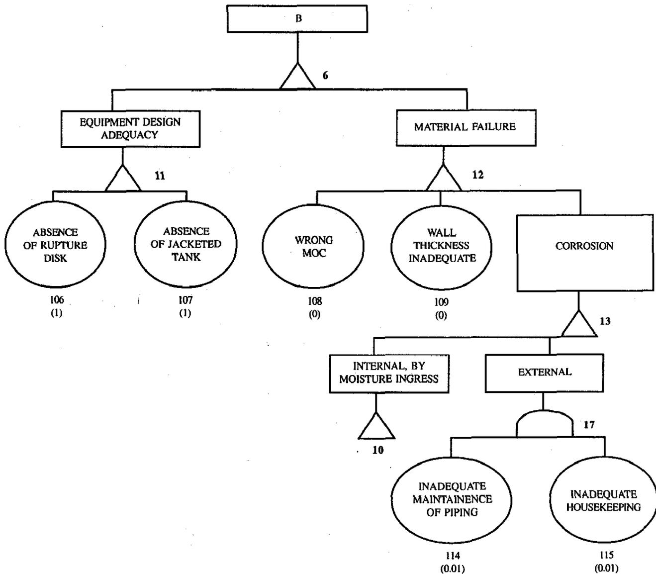
Figure 1(c). Fault tree for the release of HCl from the storage tank
