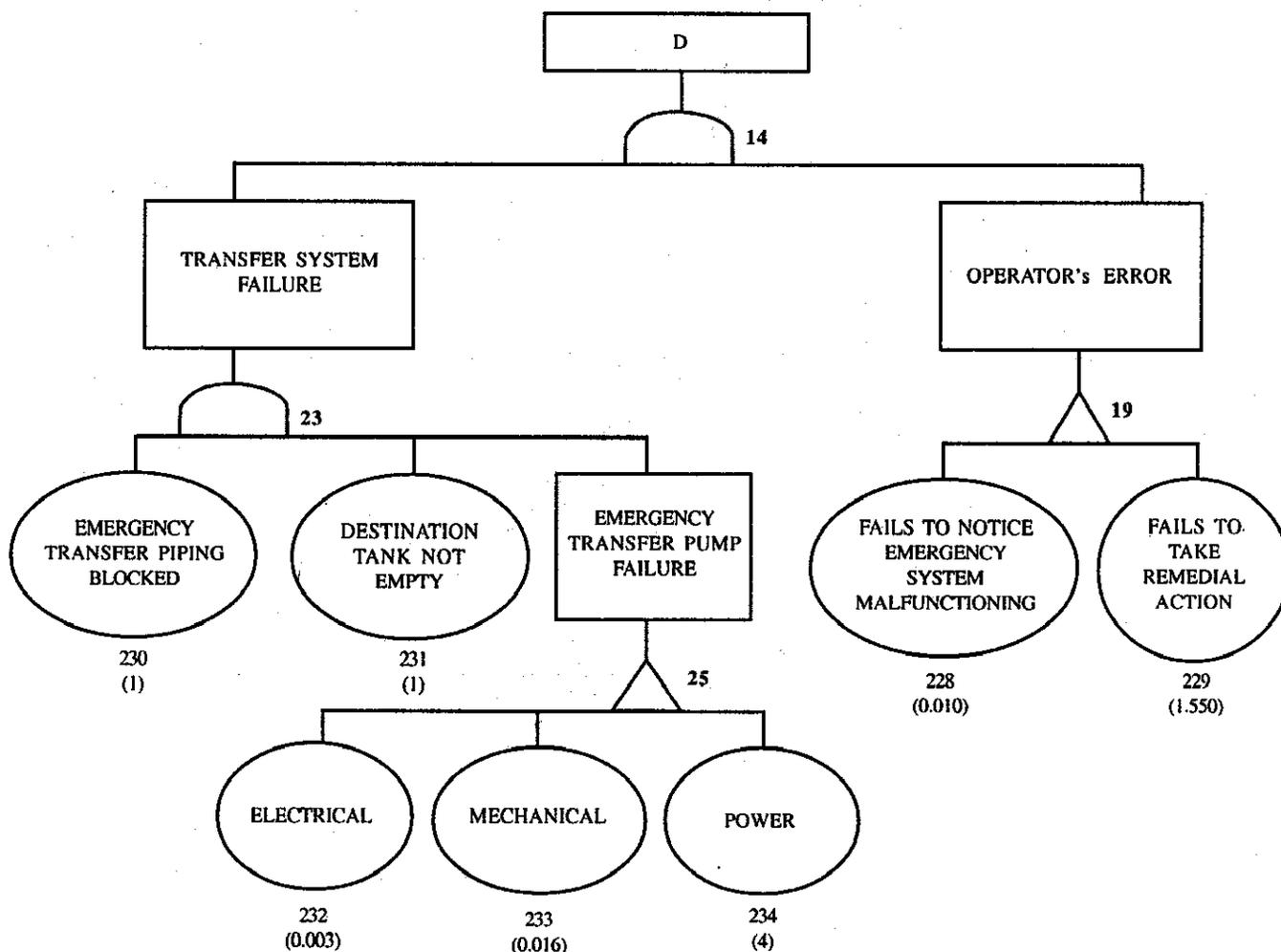
Figure 1(e). Fault tree for the release of *HCl* from the storage tank
