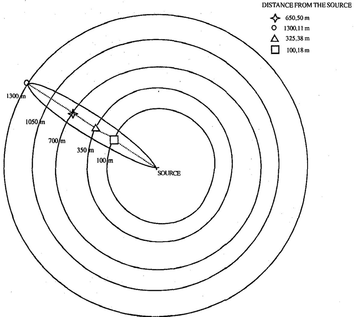
Figure 2. Depiction of an IDLH ( $145 \text{ mg/m}^3$ ) plume from the time of release to  $t = 1800 \text{ s}$  in the wind direction during monsoon
