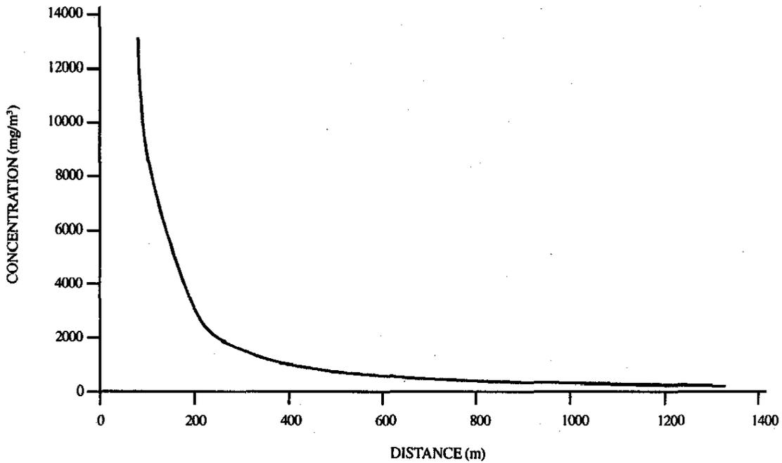
Figure 4. Variation of concentration with distance (up to IDLH limit)
