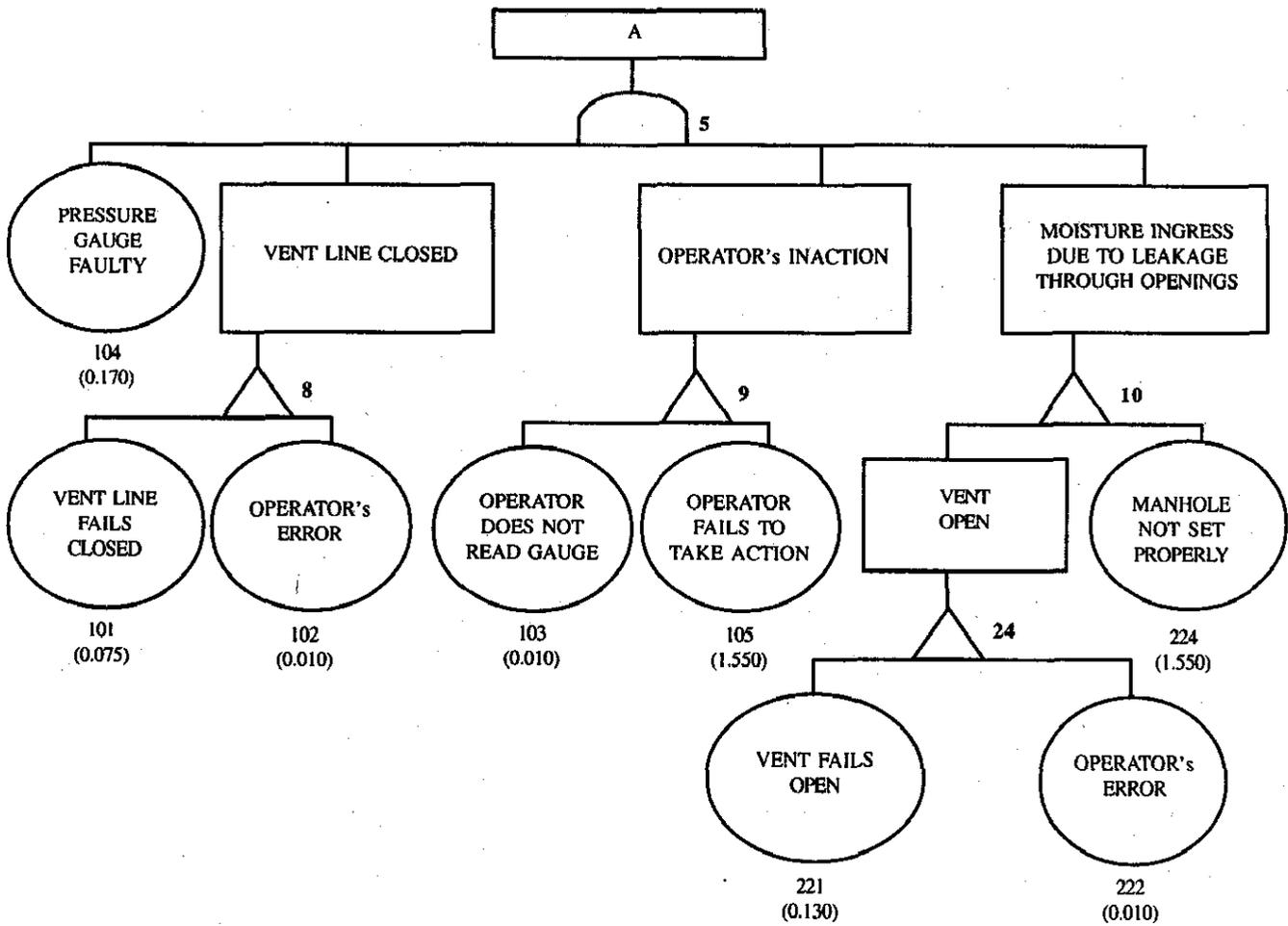
Figure 1(b). Fault tree for the release of HCl from the storage tank
