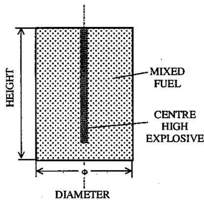
Figure 1. Section of fuel-air explosive device
