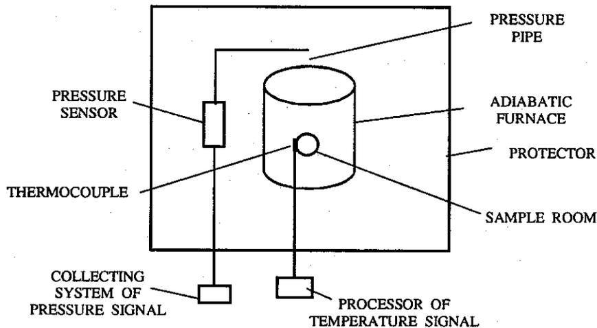
Figure 3. Testing system
