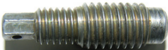
Figure 1. As received condition of the cracked pin.
