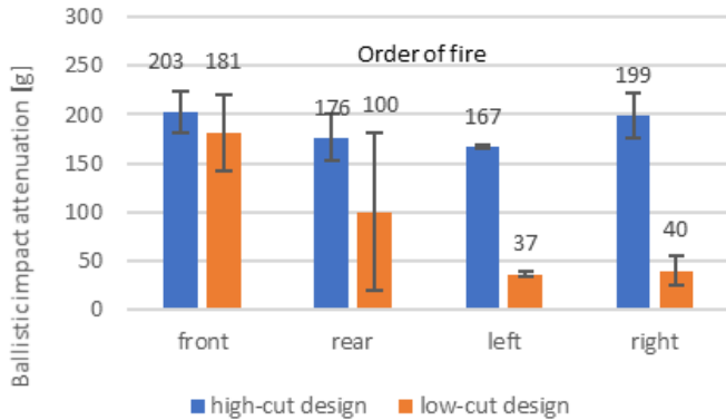
Figure 6. Ballistic impact attenuation test results of the two variants of the ballistic helmets: High-cut or low-cut helmets.
