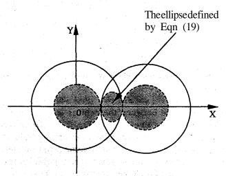
Figure 3. Effective extinction cross section wrt optimal distance between the centres of two spheres.
