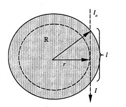
Figure 1. Effective extinction cross section of a smoke sphere
