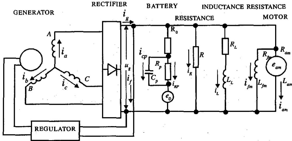
Figure 6. Schematic diagram of equivalent circuit of electrical system in military vehicle
