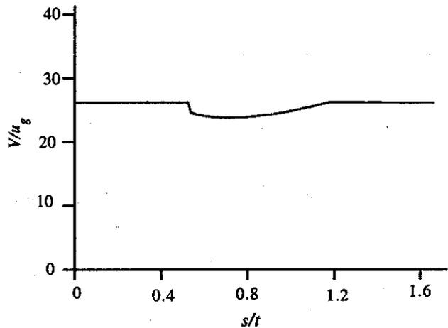
Figure 10. Surge calculated in the combined generator-battery power supply.
