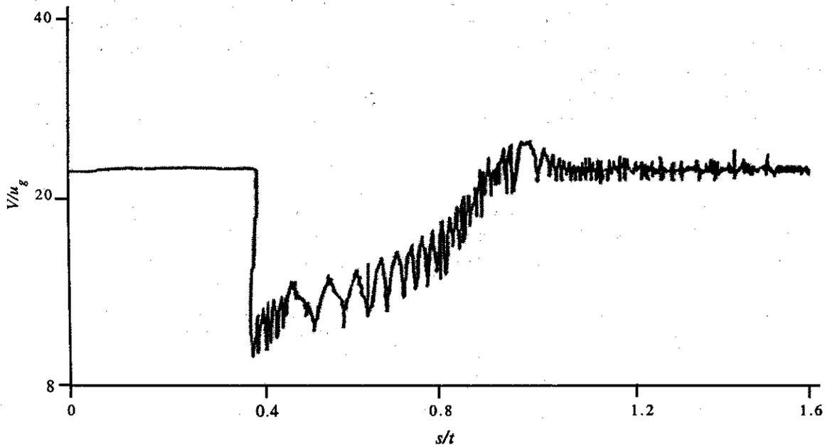
Figure 9. Surge measured when vehicle system operates with generator only, ie, no battery
