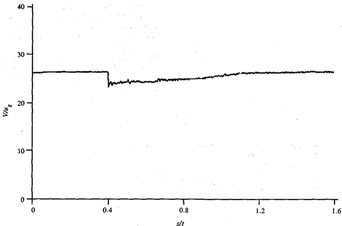
Figure 11. Surge measured in the combined generator-battery power supply
