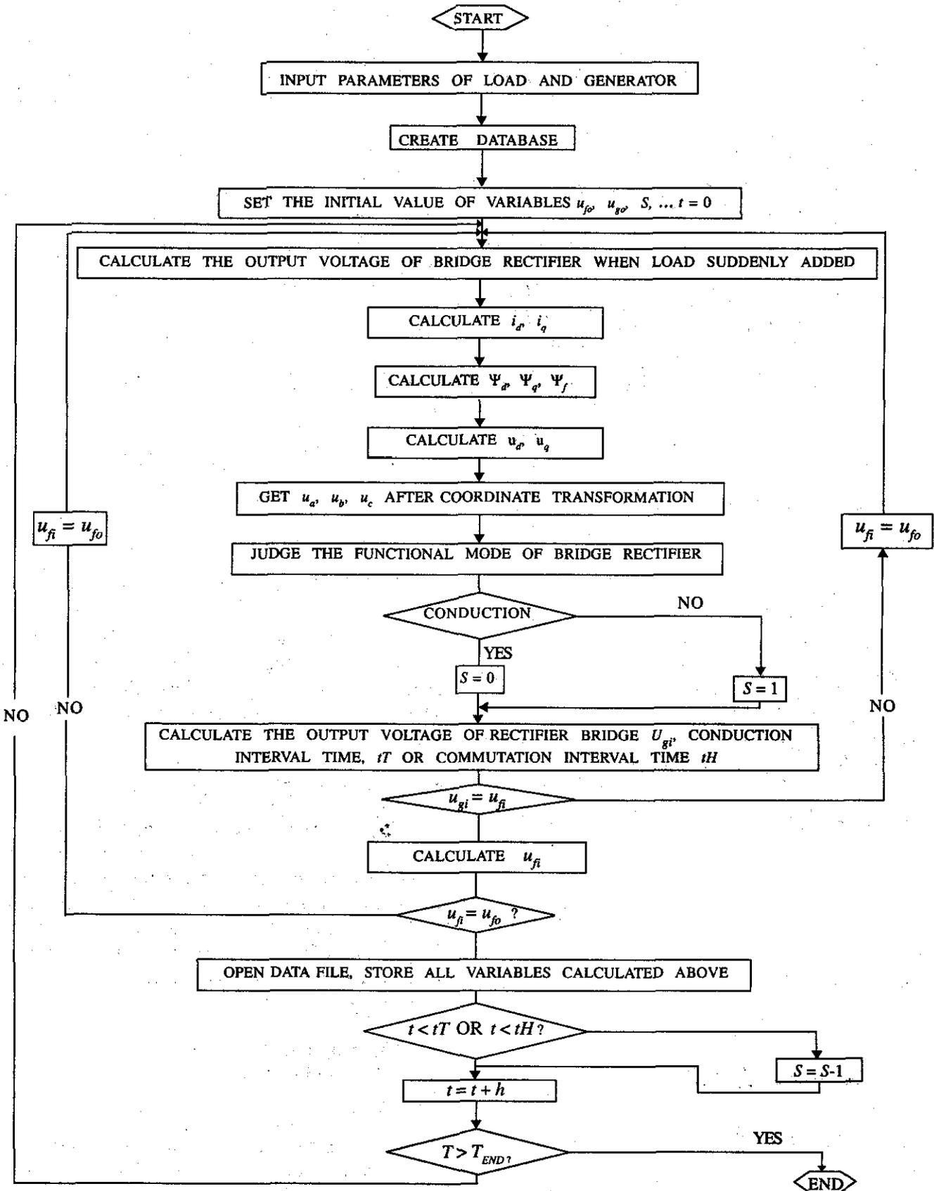
Figure 7. Program flowchart for calculation
