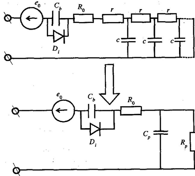
Figure 4. Equivalent circuit of the battery
