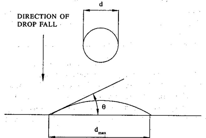
Figure 4. SPLAT formation on substrate
