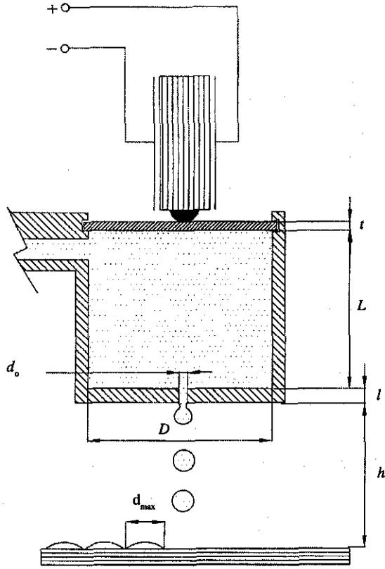
Figure 2. Piezocrystal ink-jet print head
