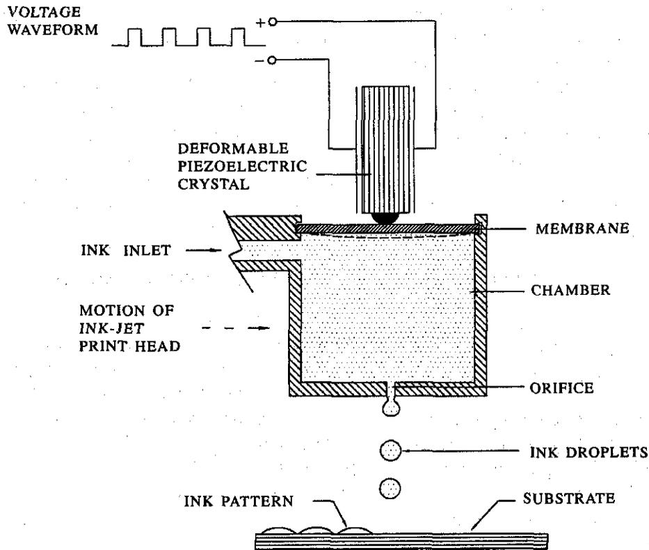
Figure 1. Schematic diagram of piezo drop-on-demand ink-jet printing system
