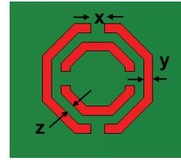
Figure 2. DS-OCSRR shaped DGS.
