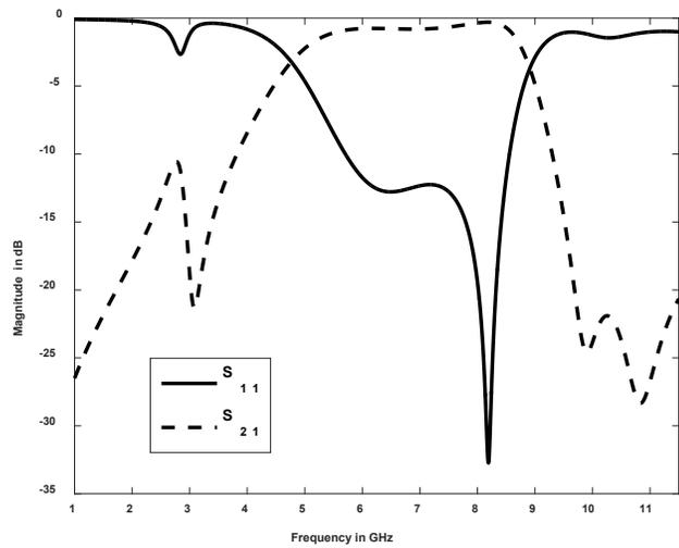
Figure 6. S-parameters of slots loaded HMSIW structure.
