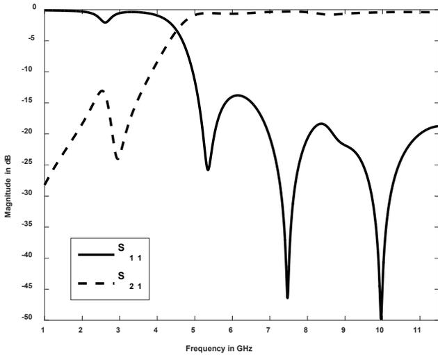
Figure 5. S-parameters of HMSIW structure.
