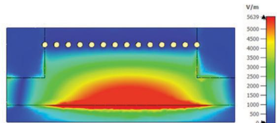
Figure 4. Electric field distribution of HMSIW structure for 6 GHz ( $f > f_c$ ).
