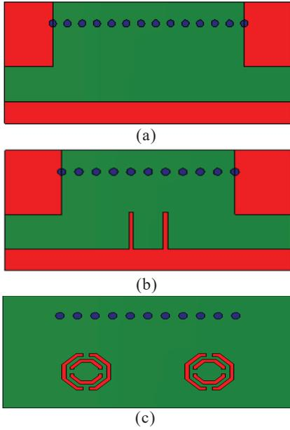
Figure 1: Evolution of the wideband HMSIW filter (a) HMSIW structure; (b) Slots in the top plane; and (c) DGS in bottom plane.
