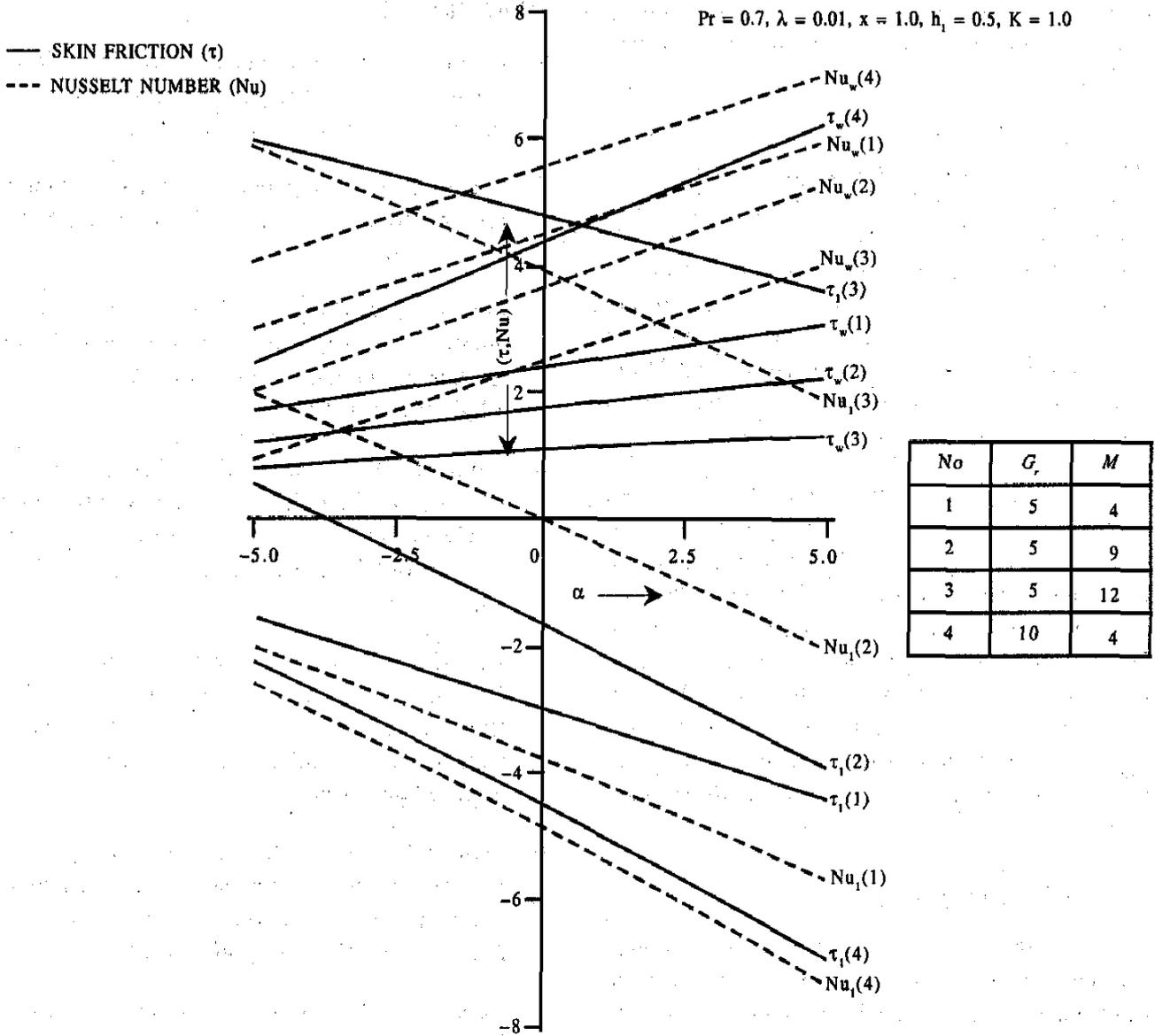
Figure 3. Skin friction ( $\tau$ ) and Nusselt number ( $Nu$ ) plotted against  $\alpha$  for different values of  $G_r$  and  $M$
