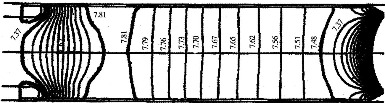
Figure 25. Stream pressure ( $\times 10^5$  Pa) contours in the combustor (with heat addition) free-stream Mach number: 2.5
