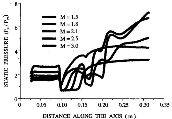
Figure 14. Static pressure distribution along the centre body
