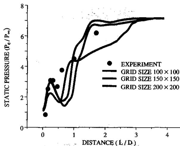
Figure 9. Cowl inner wall static pressure distribution for free-stream Mach number,  $M = 2.5$ .
