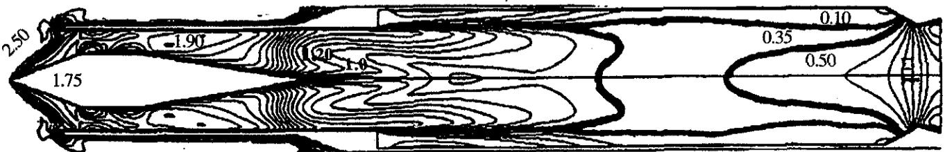
Figure 21. Mach contours—cold flow free-stream Mach number: 2.5
