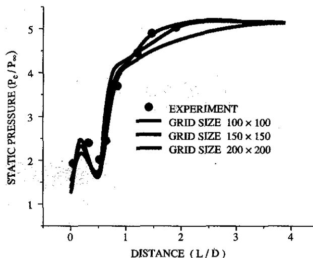
Figure 8. Cowl inner wall static pressure distribution for free-stream Mach number,  $M = 2.2$ .
