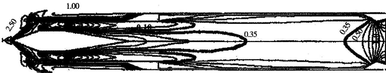
Figure 24. Mach contours with heat addition free-stream Mach number: 2.5
