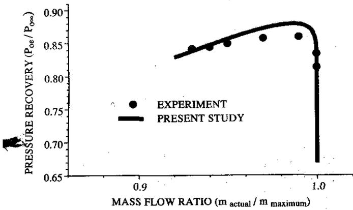
Figure 15. Air intake characteristics curve
