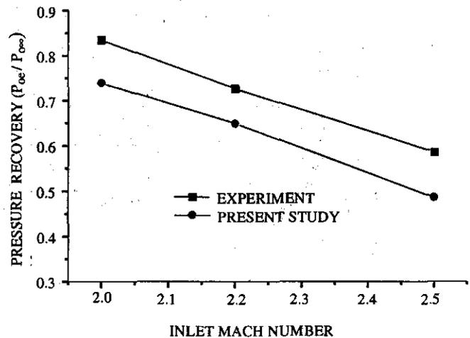
Figure 3. Variation of pressure recovery with inlet Mach number
