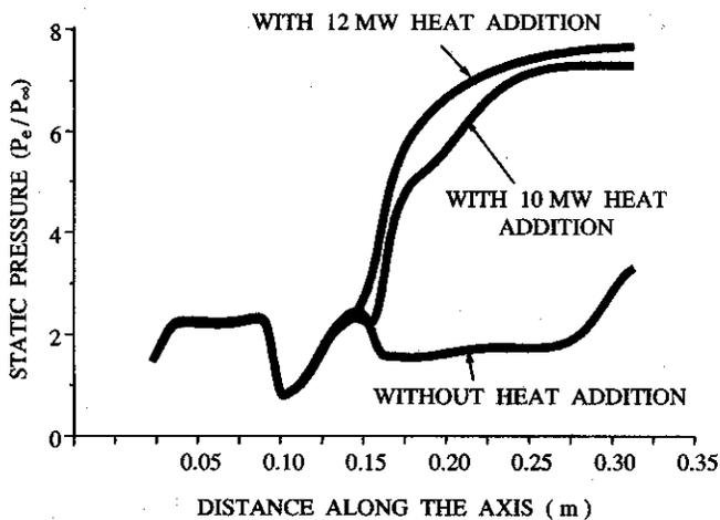
Figure 27. Effect of heat addition on the static pressure distribution along the centre body.
