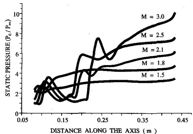
Figure 13. Static pressure distribution along the cowl inner surface.
