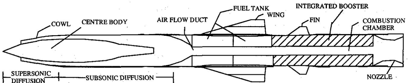
Figure 1. Schematic diagram of a typical ramjet powered flight vehicle
