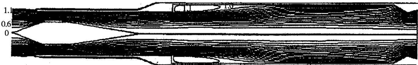
Figure 22. Stream function (kg/s) contours—cold flow free-stream Mach number: 2.5
