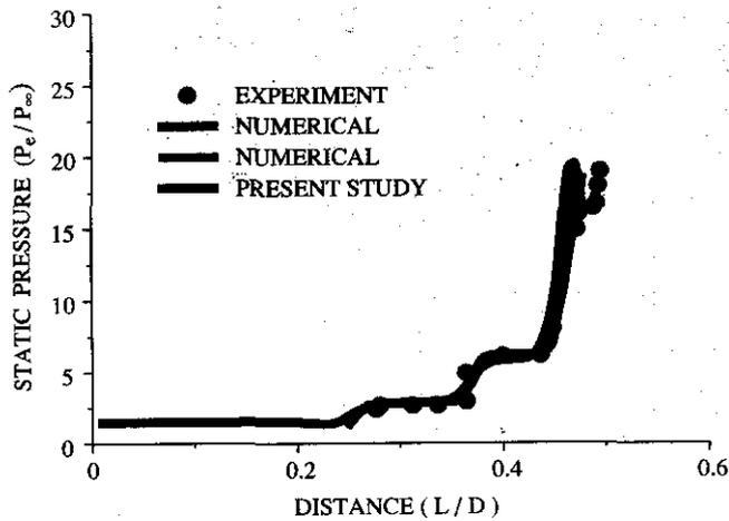
Figure 16. Static pressure distribution along cowl inner surface
