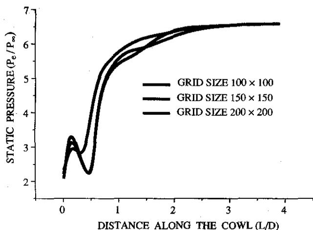
Figure 7. Static pressure distribution along the cowl inner surface.
