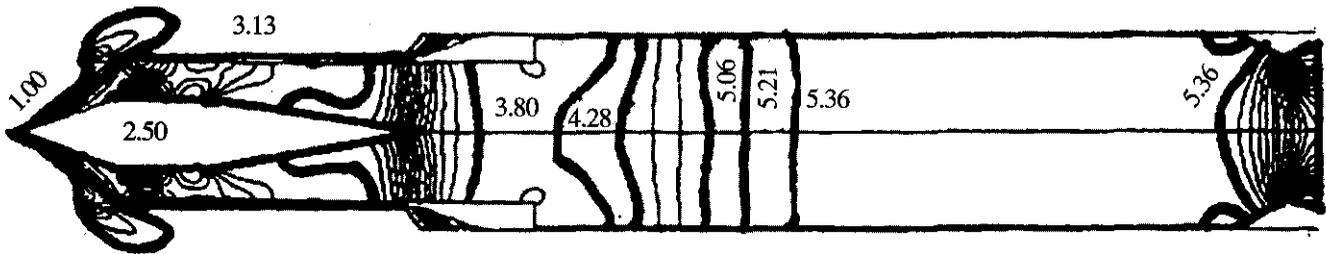
Figure 20. Static pressure ( $\times 10^5$  Pa) contours—cold flow free-stream Mach number: 2.5
