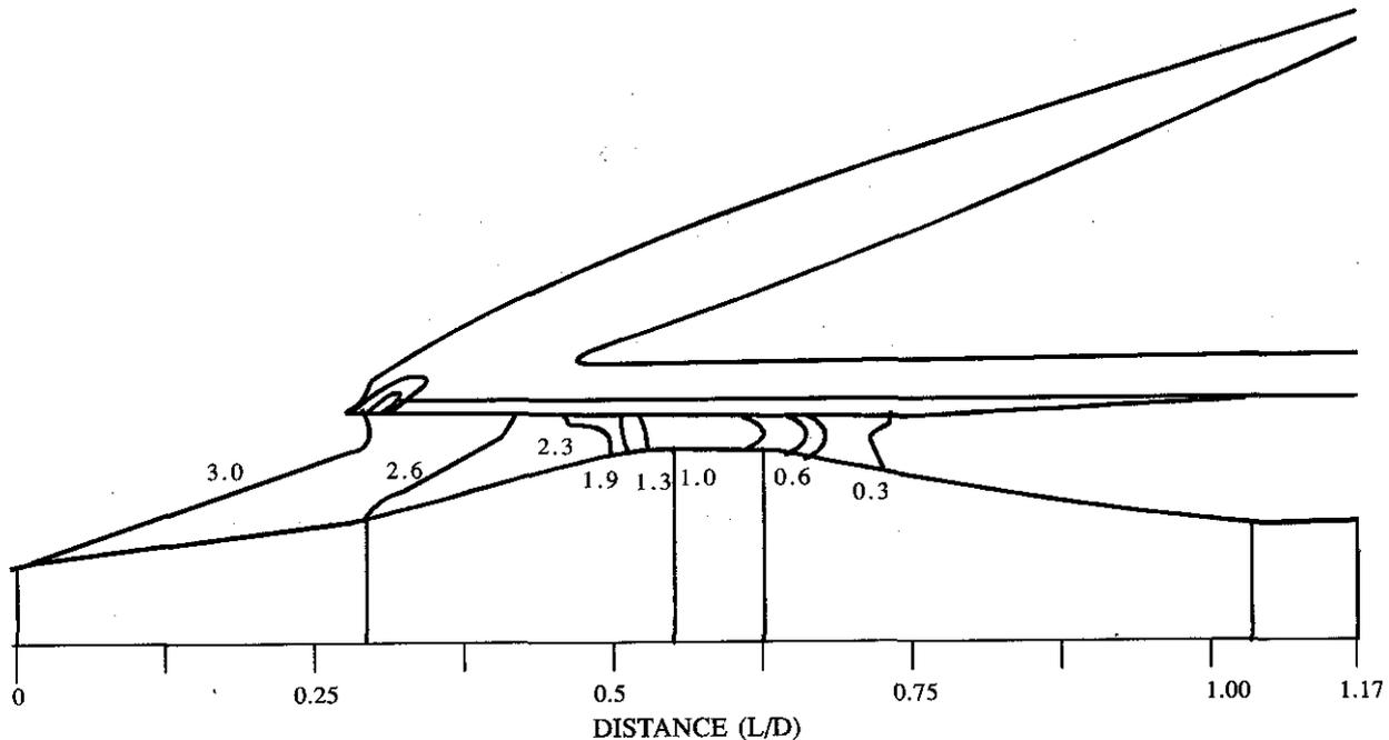
Figure 18. Mach contours for two-dimensional supersonic mixed compression air intake
