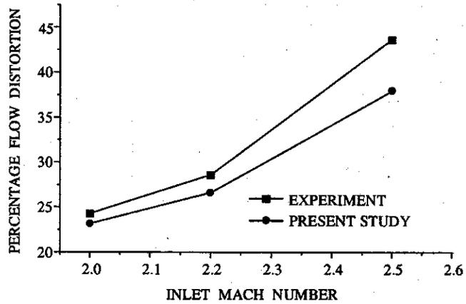
Figure 5. Flow distortion at diffuser exit for different inlet Mach number.
