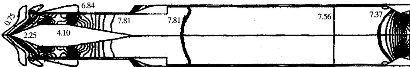
Figure 23. Static pressure ( $\times 10^5$  Pa) contours with heat addition free-stream Mach number: 2.5
