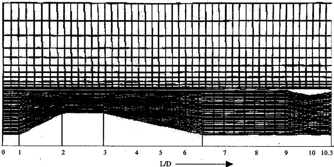
Figure 6. Typical grid employed for simulation with supersonic C-D nozzle at the exit
