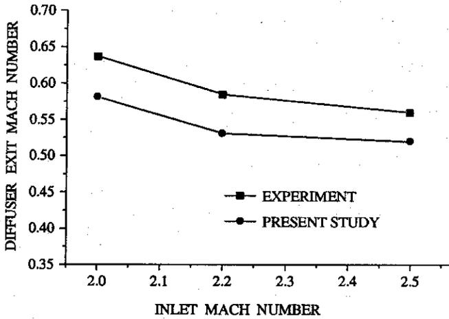
Figure 4. Variation of diffuser exit Mach number with inlet Mach number.
