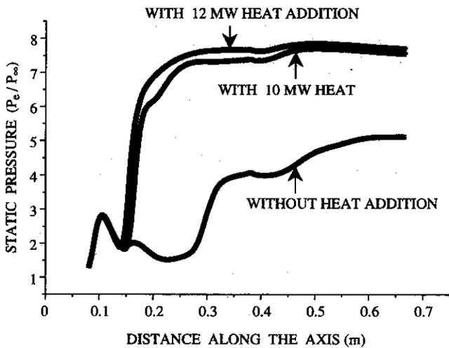
Figure 26. Effect of heat addition on the static pressure distribution along the cowl inner surface.
