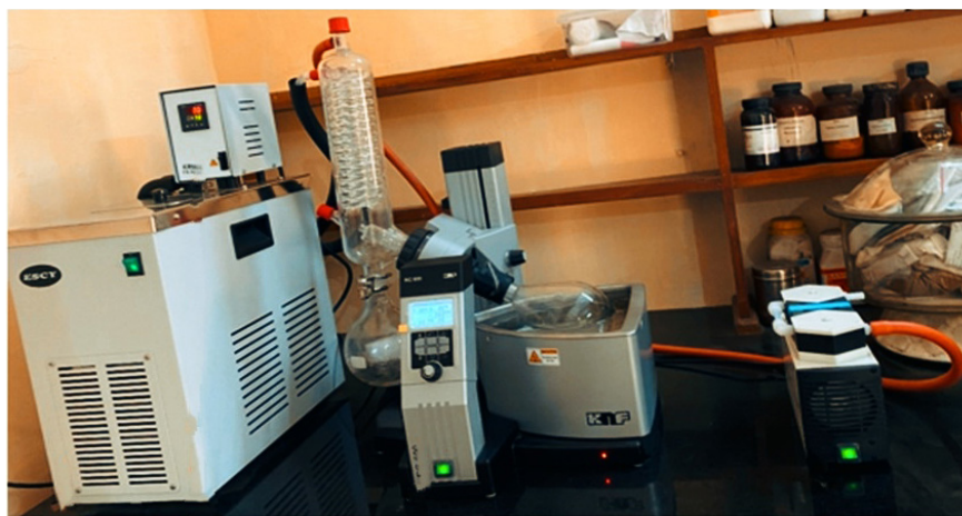
Figure 1. Rotatory evaporator used for obtaining rocket grade H_2O_2 from 50 % H_2O_2 .
