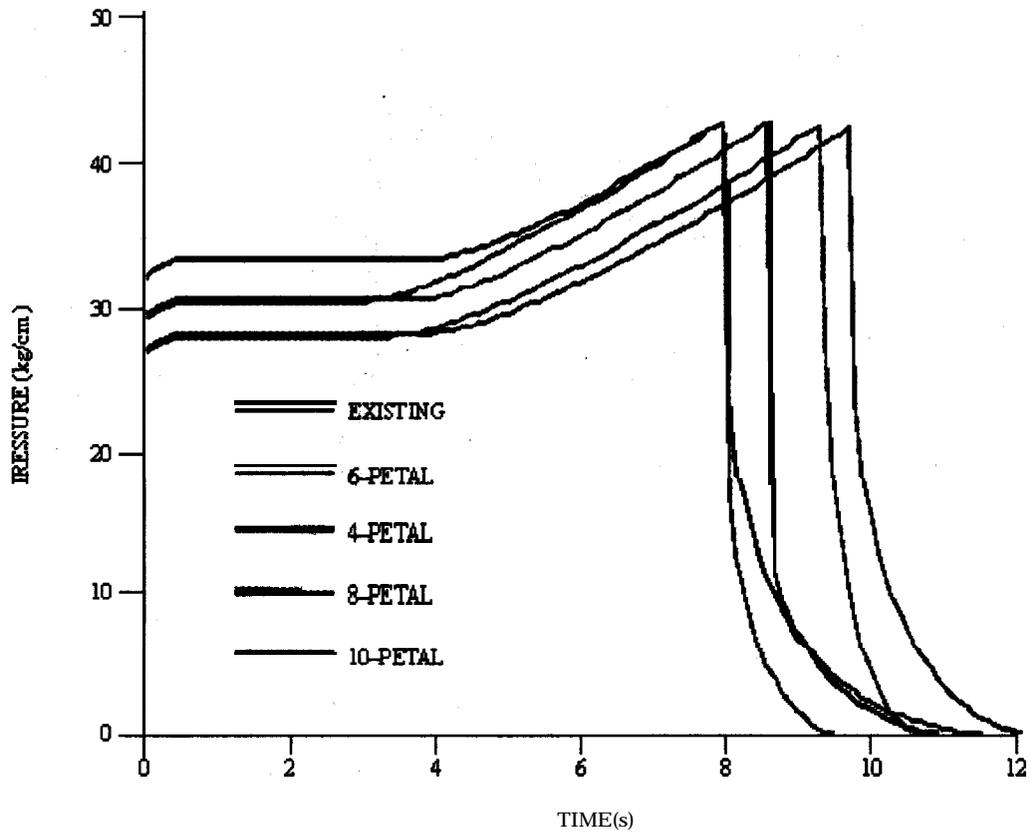
Figure 14. Comparison of pressure-time profile for different designs
