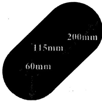
Figure 1. A 2 kg ballistic elastic motor propellant grain
