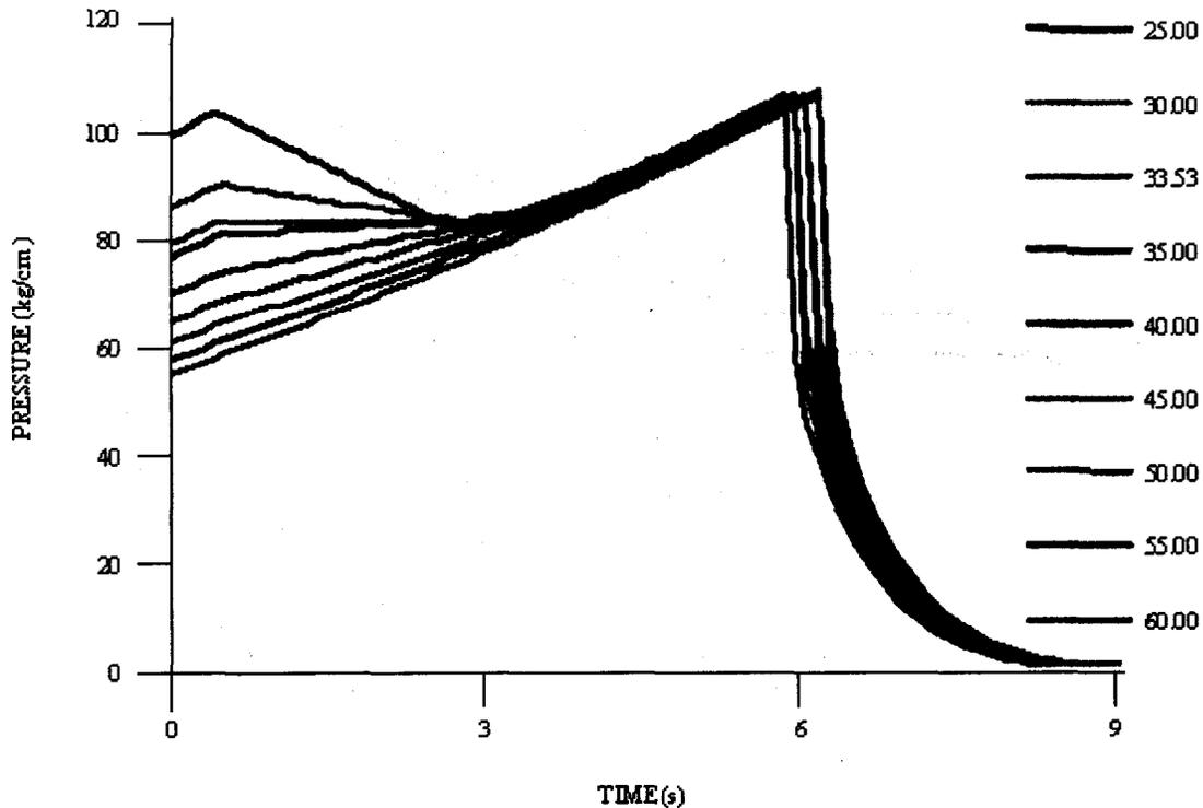
Figure 13. Parametric curve for star half-angle: Effect of variation of star half-angle
