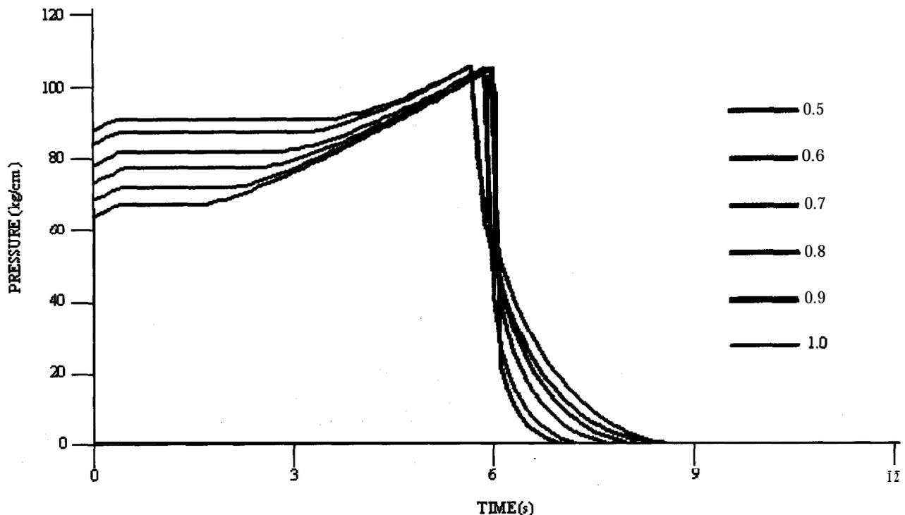
Figure 11. Parametric curve for angular fraction: Effect of variation in angular fraction
