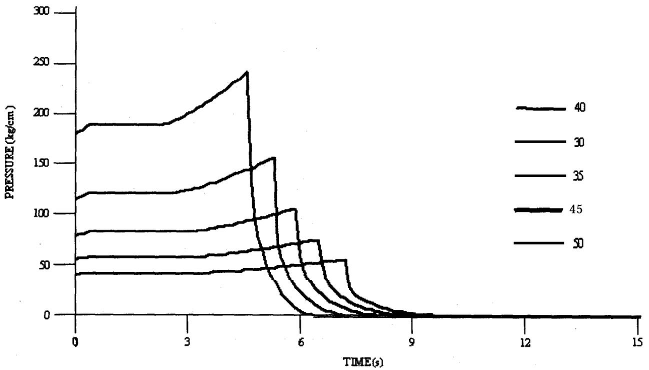
Figure 10. Parametric curve for throat diameter: Effect of variation in throat diameter
