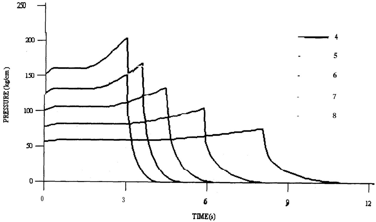
Figure 9. Parametric curve for burn rate: Effect of variation in burn rate
