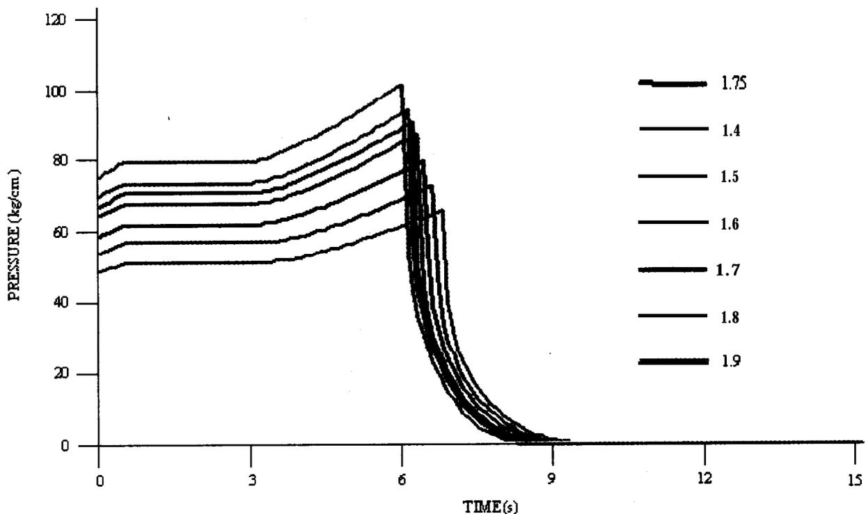
Figure 7. Parametric curve for density: Effect of variation of density of propellant
