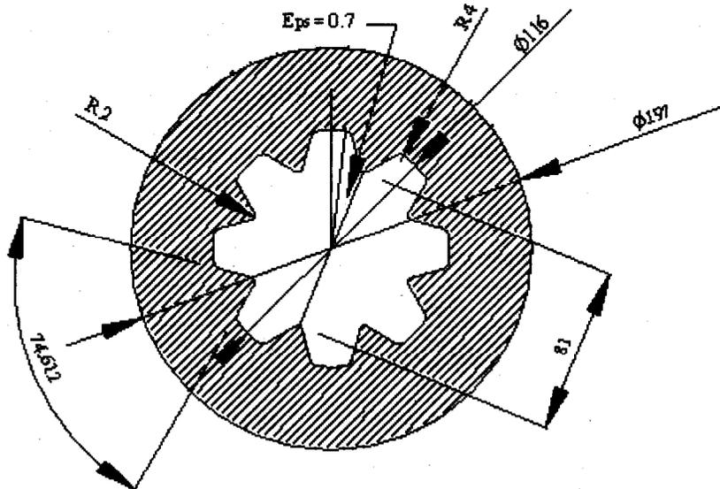
Figure 15. Proposed 40 kg ballistic evaluation motor grain cross-section
