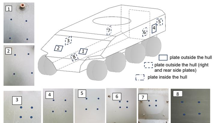
Figure 7. Distribution of the measurement areas and the points within them for the Vehicle 1.
