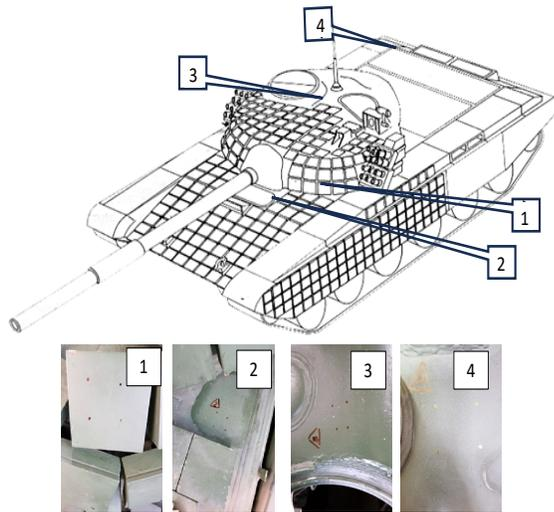
Figure 8. Distribution of the measurement areas and the points within them for the Vehicle 2.
