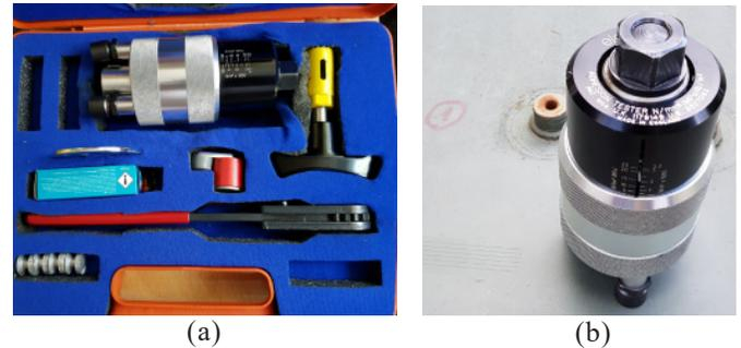
Figure 6. (a) Elcometer 106/4 tester with accessory; and (b) Tester before adhesion test.
