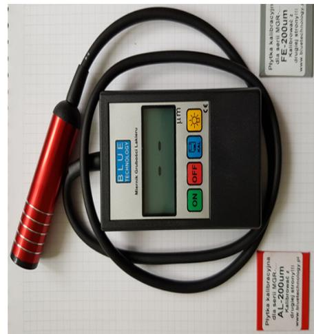
Figure 4. MGR-11-S-AL coating thickness gauge.
