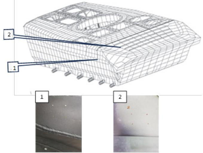
Figure 9. Distribution of the measurement areas and the points within them for the Vehicle 3.
